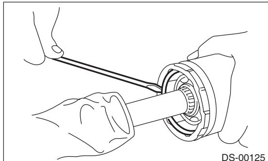
(5) Take out the DOJ outer race from the shaft assembly.
