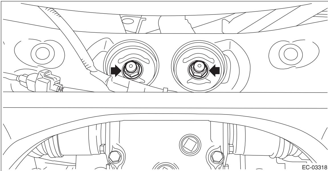
9) Remove the rear differential member from the rear sub frame assembly and the rear differential.
