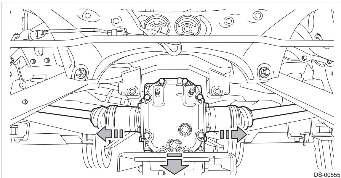
11) Remove the rear axle shaft assembly from the housing assembly - rear axle.
