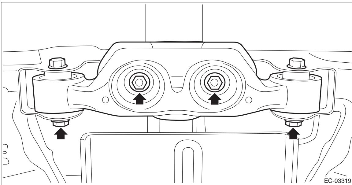
10) Completely pull out the rear axle shaft assembly while lowering the rear differential.
