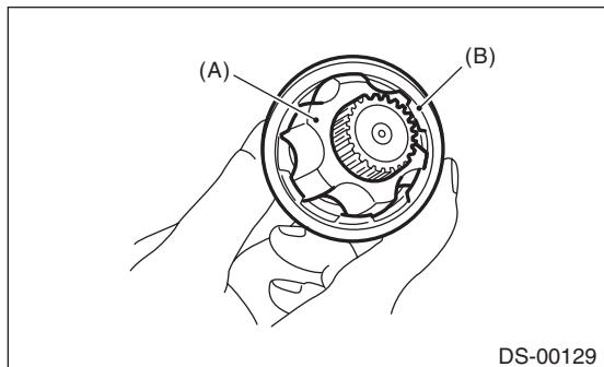
(2) Fill 80 to 90 g (2.82 to 3.17 oz) of specified grease into the inner side of the DOJ or EDJ outer race.
