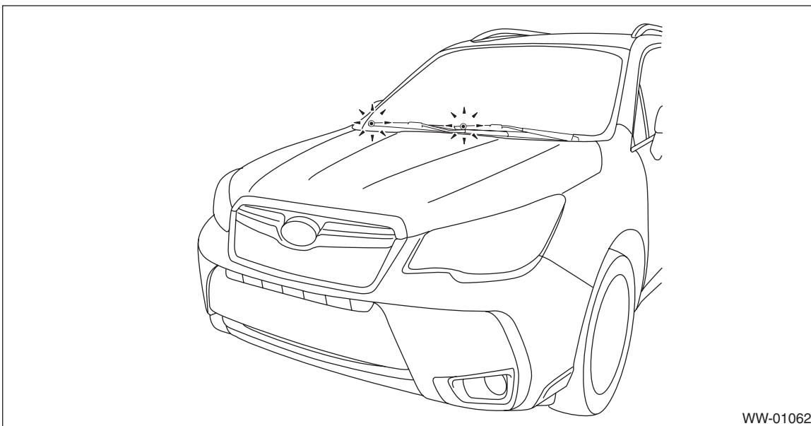
3) If the wiper blade is not aligned with the point mark, perform the removal and installation of the windshield wiper. <Ref. to WW-28, REMOVAL, Front Wiper Arm.>
