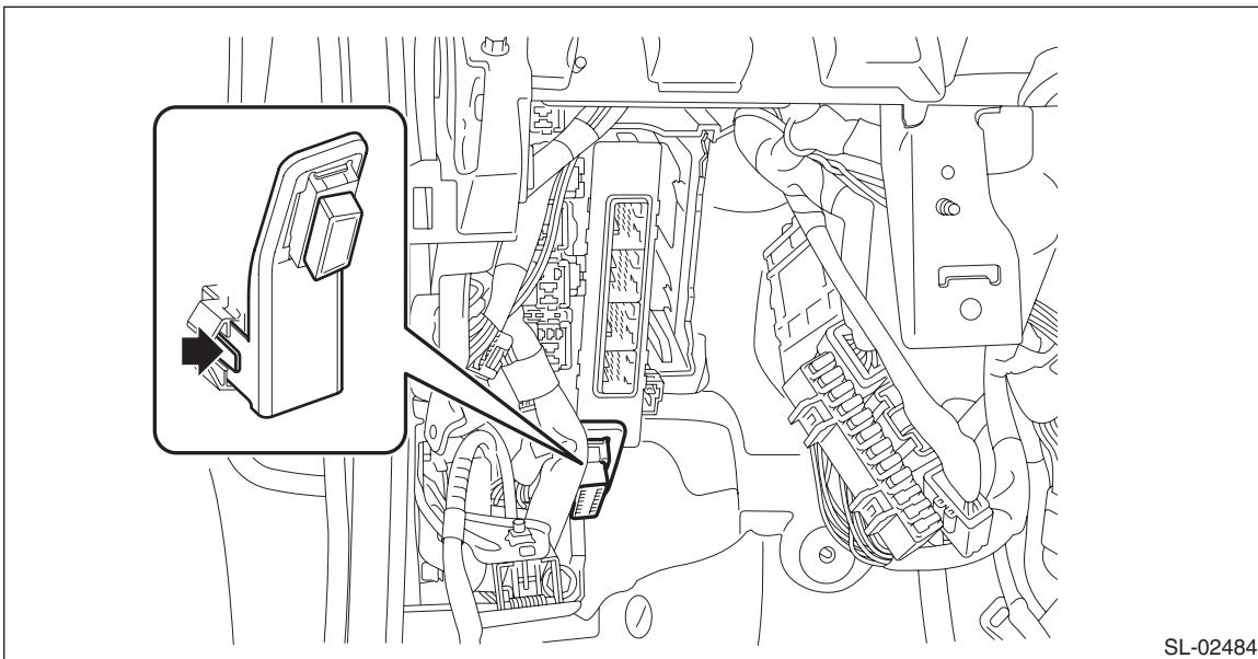
(3) Release the claws, and pull out the body integrated unit from the bracket.
