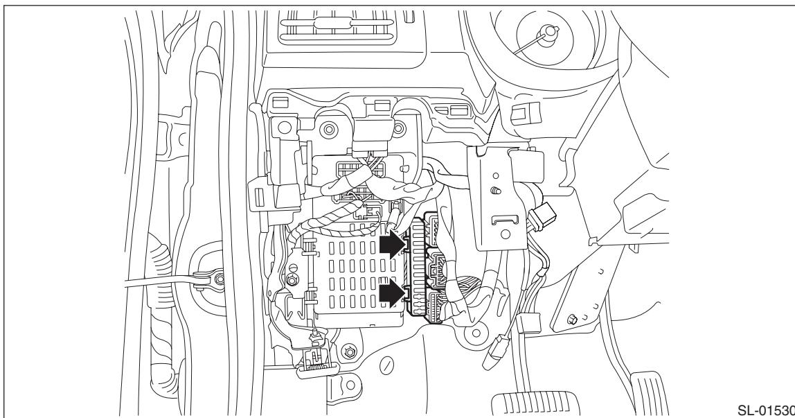
3) Remove the relay & fuse box.
