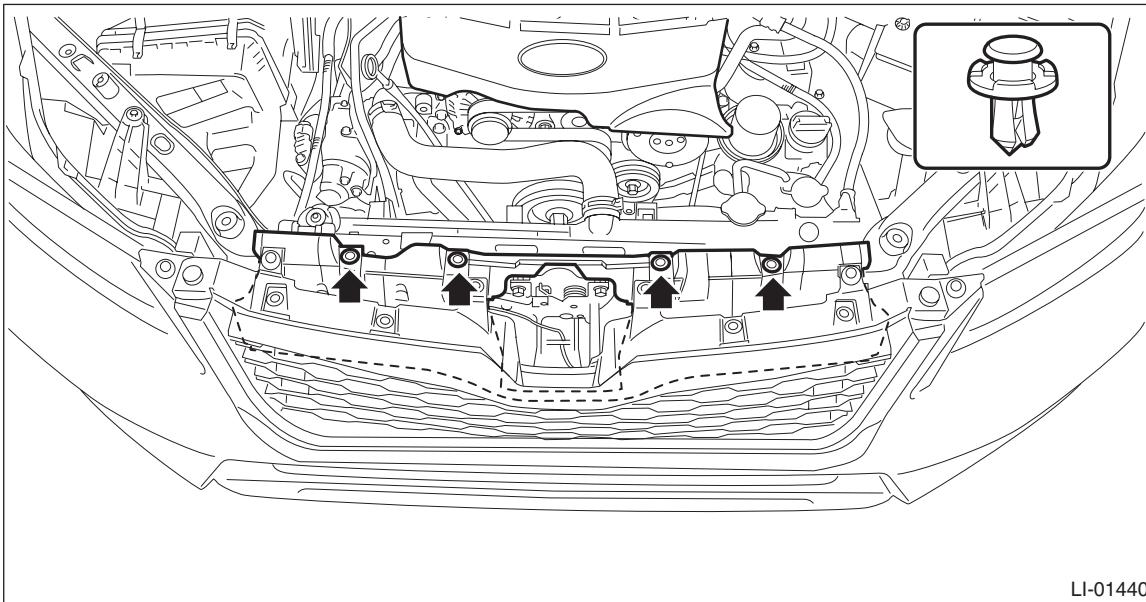
4) Remove the lock assembly - front hood.
