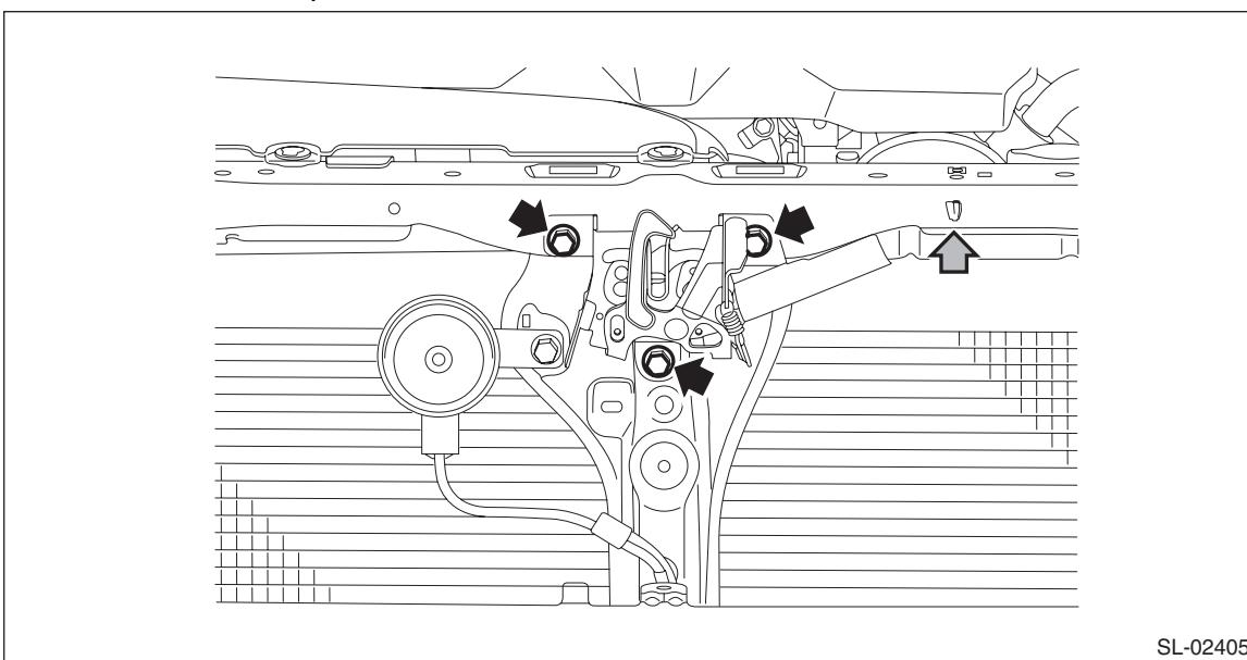
(2) Disconnect the release cable, and detach the lock assembly - front hood.
