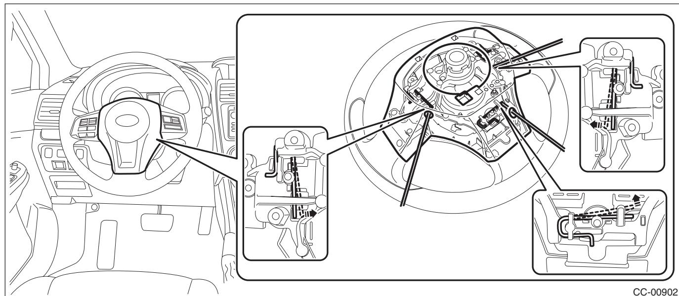
(2) Disconnect the horn harness and airbag connector, and remove the driver's airbag module. <Ref. to AB-21, DRIVER'S AIRBAG MODULE, KNEE AIRBAG MODULE, CURTAIN AIRBAG MODULE AND PRETENSIONER, PROCEDURE, Airbag Connector.>
