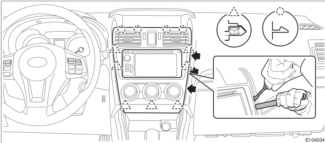
3) Release the claws, and then remove the grille assembly - CTR ventilation from the panel center assembly.
