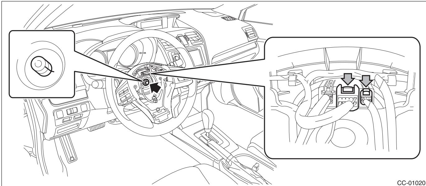
6) Remove the cruise control command switch assembly.
