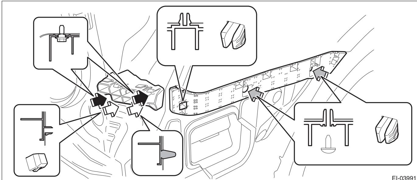
6) From behind the bumper face - rear, release the nuts and claws and remove the reflex reflector assembly.
