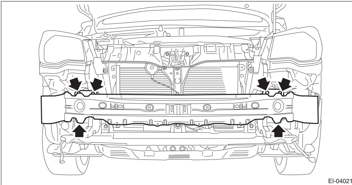
4) Remove the bolt, and then detach the front sub sensor. <Ref. to AB-22, FRONT SUB SENSOR, FRONT DOOR IMPACT SENSOR AND SATELLITE SAFING SENSOR, PROCEDURE, Airbag Connector.>
