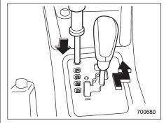
If you inadvertently have turned the ignition switch to the "LOCK" position with the selector lever in the "N" position, proceed as follows. To remove the shift lock release cover, refer to the "Shift lock release" section in this chapter. Then, with a screwdriver inserted into the hole, move the selector lever to the "P" position. If the selector lever reverse inhibiting function fails, have the vehicle inspected by the nearest SUBARU dealer.
