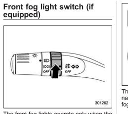
The front fog lights operate only when the low beam headlights are illuminated.
