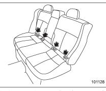
The lower anchorages (bars) are used for installing a child restraint system only on the rear seat window-side seating positions. For each window-side seating position, two lower anchorages are provided. Each lower anchorage is located where the seat cushion meets the seatback.
