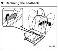
Pull the reclining lever up and adjust the seatback to the desired position. Then release the lever and make sure the seatback is securely locked into place.
