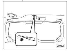
1. Remove the plug on the roof trim of the cargo area by inserting the end of the flathead screwdriver between the roof and plug and prying it off.
