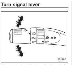
To activate the right turn signal, push the turn signal lever up. To activate the left turn signal, push the turn signal lever down. When the turn is finished, the lever will return automatically. If the lever does not return after cornering, return the lever to the neutral position by hand.
