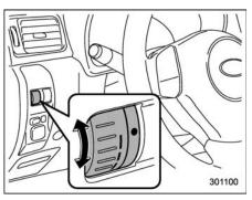
The brightness of clock display, audio, air conditioner, information display and instrument panel illumination dims when the light switch is in the "zooz" or " $\equiv$ O" positions. You can adjust brightness of the instrument panel illumination for better visibility.
