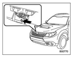
Release the secondary hood release by moving the lever between the front grille and the hood toward the left.
