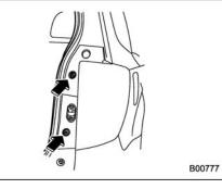
1. Using a Phillips screwdriver, remove the upper and lower screws that secure the rear combination light assembly.
