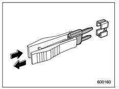
Pull out the fuse with the fuse puller.
