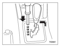
4. Insert the screwdriver into the hole.
