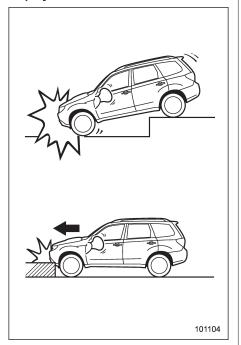
Only the driver's SRS frontal airbag or both driver's and front passenger's SRS frontal airbags may be activated when the vehicle sustains a hard impact in the undercarriage area from the road surface (such as when the vehicle plunges into a deep ditch, is severely impacted or knocked hard against an obstacle on the road such as a curb).
