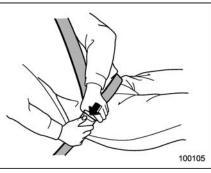
Push the button on the buckle. Before closing the door, make sure that the belts are retracted properly to avoid catching the belt webbing in the door.
