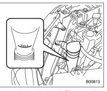
Remove the washer tank filler cap, then check the fluid level indicated by the level gauge (attached to the inside of the cap). If the level is near the "Low" mark, add fluid until it reaches the "Hi" level on the
