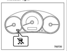
This single light has the function of indicating malfunctions in the Vehicle Dynamics Control system and the function of indicating that the Vehicle Dynamics Control system is not operating. It illuminates in the event of a malfunction in the system and is illuminated whenever the system is not operating.
