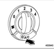
The air conditioner operates only when the engine is running.
