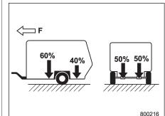
the rear axle of the towing vehicle. This may cause the rear wheels to skid, especially during braking or when vehicle speed is reduced during cornering, resulting in oversteer, spin out and/or jackknifing.
