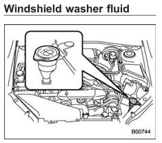
If you spray washer fluid on the windshield but the supply of washer fluid appears to diminish, check the level of washer fluid in the tank.
