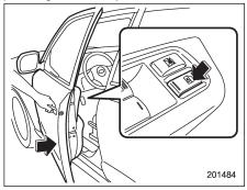
6. Push the front side ("LOCK" side) of the power door locking switch to set the door locks.
