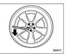
6. Loosen the wheel nuts using the wheel nut wrench but do not remove the nuts.
