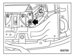
2. Place a proper container under the drain plug and loosen the drain plug.
