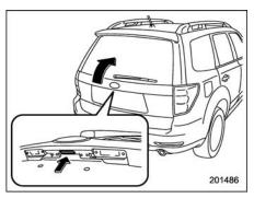
The rear gate can be locked and unlocked using either the remote keyless entry system or the power door locking switches.
