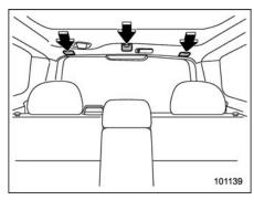
The tether anchorages (upper anchorages) are provided at the locations shown in the above illustration.
