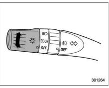
To turn on the headlights, turn the knob on the end of the turn signal lever.
