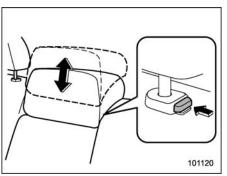
To raise the head restraint, pull it up while pressing the release button on the top of the seatback.
