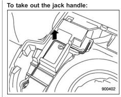
Open the floor cover of the cargo area, and take out the jack handle. To take out the jack and wheel nut wrench:
