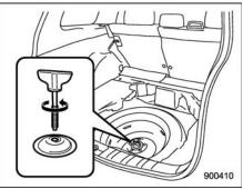
Turn the attaching bolt counterclockwise, then take the spare tire out.
