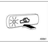
**ON position (Recirculation):** Interior air is recirculated inside the vehicle. Push the air inlet selection button to the ON position. The indicator light will illuminate.
