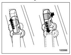
The shoulder belt anchor height should be adjusted to the position best suited for the driver/front passenger.
