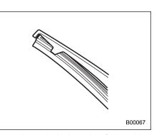
Securely retain both ends of the rubber with the stoppers on the plastic support ends. If the rubber is not retained properly, the wiper may scratch the rear window glass.
