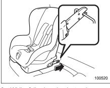
2. While following the instructions supplied by the child restraint system manufacturer, connect the lower hooks onto the lower anchorages located at "©" marks on the bottom of the rear seatback. When the hooks are connected, make sure the adjacent seatbelts are not caught.
