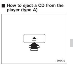
When a disc is being played back or when a disc is in the player, press the eject button "**A**". The disc will be ejected.
