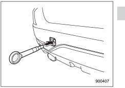
3. Screw the towing hook into the thread hole until its thread can no longer be seen.
