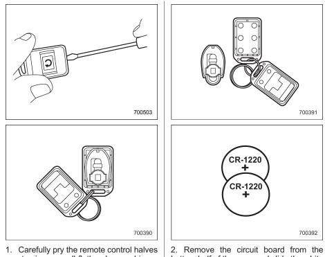
apart using a small flathead screwdriver. bottom half of battor battor
