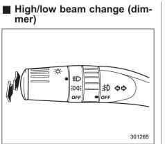
To change from low beam to high beam, push the turn signal lever forward. When the headlights are on high beam, the high beam indicator light "and the combination meter is also on.
