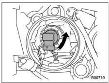
Remove the bulb from the headlight assembly by turning it counterclockwise.
