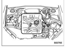
2. Pull out the level gauge that has the "">"" symbol on top, wipe it clean, and insert it again.
