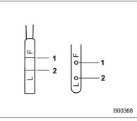
Pull out the level gauge again and check the oil level on it. If it is below the
