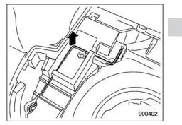
The jack handle is stored under the floor cover of the cargo area.
