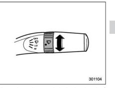
When the wiper switch is in the " $\nabla$ " position, turn the dial to adjust the operating interval of the wiper.
