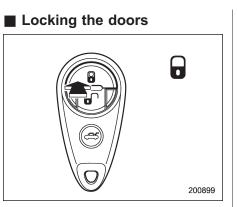
Press the """ button to lock all doors and the rear gate. An electronic chirp will sound once and the turn signal lights will flash once.
