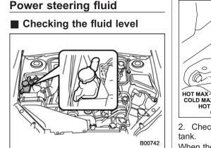
The power steering fluid expands greatly as its temperature rises; the fluid level differs according to fluid temperature. Therefore, the reservoir tank has two different checking ranges for hot and cold fluids.
