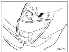
6. Put the rear combination light assembly into place while aligning the clip with the guide on the vehicle.
