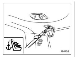
8. If the child restraint system requires a top tether, latch the hook onto the top tether anchorage and tighten the top tether. Refer to "Top tether anchorages" in this section for additional instructions.
