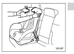
6. Before having a child sit in the child restraint system, move it back and forth and right and left to check if it is firmly secured. Sometimes a child restraint can be more firmly secured by pushing it down into the seat cushion and then tightening the seatbelt.
