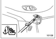
Attach the child restraint top tether hook to the appropriate upper anchorage.
