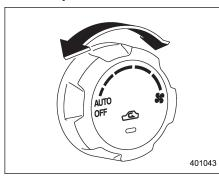
The fan operates only with the ignition switch in the ON position. The fan speed control dial is used to select the AUTO (automatic control) mode or to select the desired fan speed. The dial's positions and their functions are as follows:
