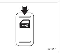
5. Before the electronic tone stops sounding, push the lock side of the power door lock switch the same number of times as the leftmost digit of the transmitter code. For example, push the lock switch eight times if the leftmost digit of the code is 8.
