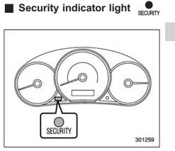
The security indicator light deters potential thieves by indicating that the vehicle is equipped with an immobilizer system. It begins flashing (approximately once every 3 seconds) approximately 60 seconds after the ignition switch is turned from the "ON" position to the "Acc" or "LOCK" position or immediately after the key is pulled out.
