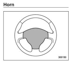
To sound the horn, push the horn pad.
