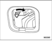
3. Turn the lever to the right position using a screwdriver.
