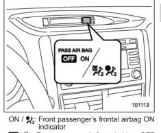
off / ⅔: Front passenger's frontal airbag OFF indicator
