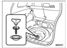
14. Store the flat tire in the spare tire compartment. Put in the spacer and tighten the attaching bolt firmly. Also store the jack, jack handle and wheel
