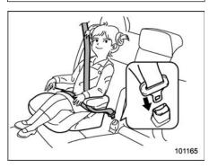
1. Place the booster seat in the rear seating position and sit the child on it. The child should sit well back on the booster
