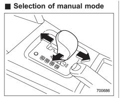
With the vehicle either moving or stationary, move the selector lever from the "D" position to the manual gate then move it to the "+" end or "–" end of the manual gate to select manual mode.
