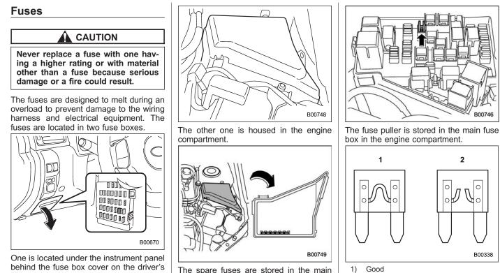
behind the fuse box cover on the driver's seat side. To remove the cover, pull it out.
