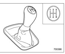
The manual transmission is a fully synchromeshed, 5-forward-speed and 1-reverse-speed transmission.
