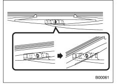
2. Turn the wiper blade assembly counterclockwise.
