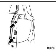
7. Tighten the upper and lower screws.
