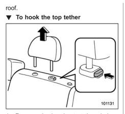
1. Remove the headrest at the windowside seating position where the child restraint system has been installed with the lower anchorages or seatbelt; lift up the headrest while pressing the release button. Store the headrest in the cargo area. Avoid placing the headrest in the passenger compartment to prevent it from being thrown around in the passenger compartment in a sudden stop or a sharp turn.
