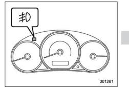
The indicator light located on the combination meter will illuminate when the front fog lights are on.
