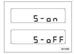
It is possible to activate or deactivate the movement of the meter needles and gauge needles that takes place when the ignition switch is turned to the "ON" position.
