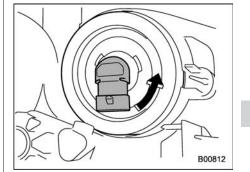
Remove the bulb from the headlight assembly by turning it counterclockwise.
