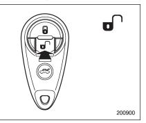
Press the "n" button to unlock the driver's door. An electronic chirp will sound twice and the turn signal lights will flash twice. To unlock all doors and the rear gate, briefly press the "n" button a second time within 5 seconds.
