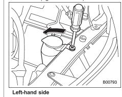
2. Use a screwdriver to remove the secured clip of the washer tank. To make it easy to access the bulb, move the washer tank to the horizontal direction (left-hand side).
