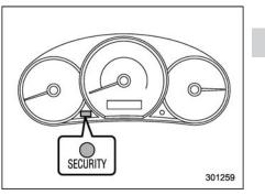
The security indicator light deters potential thieves by indicating that the vehicle is equipped with an immobilizer system. It begins flashing (approximately once every 3 seconds) approximately 60 seconds after the ignition switch is turned from the "ON" position to the "Acc" or "LOCK" position or immediately after the key is pulled out.
