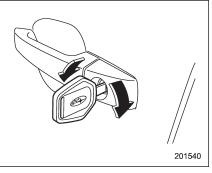
To lock the driver's door from the outside with the key, turn the key toward the rear. To unlock the door, turn the key toward the front.
