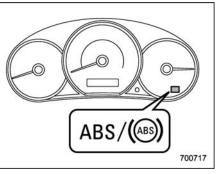
The ABS warning light illuminates when the ignition switch is turned to the "ON" position and turns off after approximately 2 seconds.
