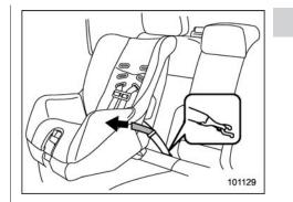
3. [If your child restraint system is of a flexible attachment type (which uses tether belts to connect the child restraint system properly to the lower anchorages)] While pushing the child restraint into the seat cushion, pull both left and right lower tether belts up to secure the child restraint system firmly by taking up the slack in the belt.
