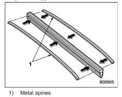
3. If the new blade rubber is not provided with two metal spines, remove the metal spines from the old blade rubber and install them in the new blade rubber.
