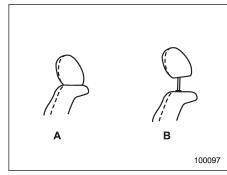
A) When not used (retracted position)B) When used (click position)
