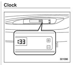
The clock shows the time while the ignition switch is in the "Acc" or "ON" position.
