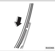
4. Align the claws of the plastic support with the grooves in the blade rubber assembly, then slide the blade rubber assembly into place.
