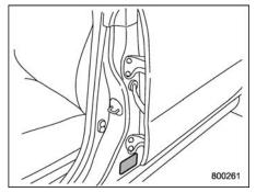
The certification label attached to the driver's side doorjamb shows GVWR (Gross Vehicle Weight Rating) and GAWR (Gross Axle Weight Rating).
