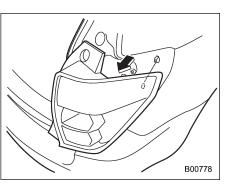
2. Slide the rear combination light assembly rearward and remove it from the vehicle.
