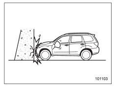
A head-on collision against a thick concrete wall at a vehicle speed of 12 to 19 mph (20 to 30 km/h) or higher activates only the driver's SRS frontal airbag or both driver's and front passenger's SRS frontal airbags. The airbag(s) will also be activated when the vehicle is exposed to a frontal impact similar in fashion and magnitude to the collision described above.
