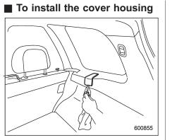
1. Remove the cover of the retainers by prying on the edge with a flat-head screwdriver.
