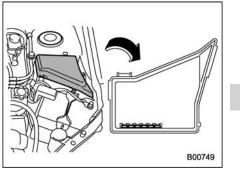
2. Pull any one spare fuse out of the spare fuse holder in the engine compartment. Spare fuses are attached on the back side of the fuse holder cover. You may pick up any one fuse in the spare fuse holder.
