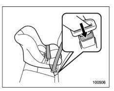
8. To remove the child restraint system, press the release button on the seatbelt buckle and allow the belt to retract completely. The belt will return to the ELR mode.
