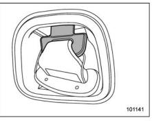
2. Allow the retractor to roll up the belt.
