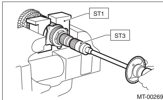
4) If the starting torque is not within the specified limit, select new adjusting washer No. 1 and recheck starting torque.
