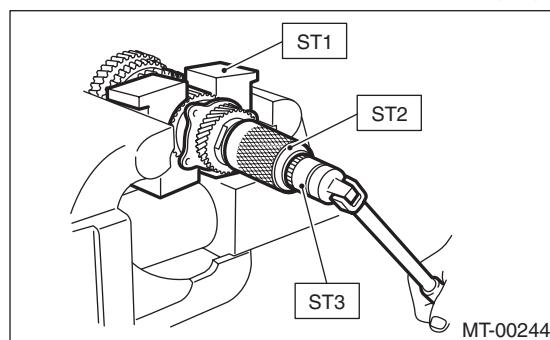
2) Draw out the drive pinion from driven shaft. Remove the differential bevel gear sleeve, adjusting washer No. 1, adjusting washer No. 2, thrust bearing, needle bearing and drive pinion collar.
