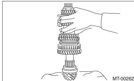
13) Install the drive pinion collar, needle bearing, adjusting washer No. 2, thrust bearing, adjusting washer No. 1 and differential bevel gear sleeve in this order.
