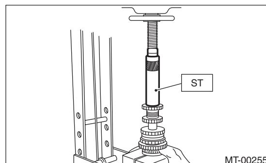
7) Install a set of roller bearings onto the driven shaft using ST and a press.
