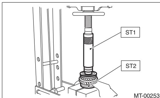
5) Install the 2nd driven gear, inner baulk ring, synchro cone and outer baulk ring, and insert them onto driven shaft.
