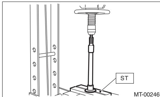
4) Unlock the crimping of lock nut. Remove the lock nut using ST1 and ST2.
