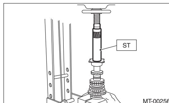
8) Position the woodruff key in groove of the rear of driven shaft. Install the 5th driven gear onto driven shaft using ST and a press.
