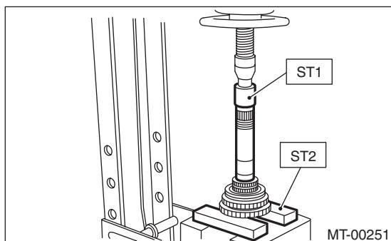
11) Remove the sub gear, washer, and snap ring (outer) for the 1st driven gear. (Non-turbo model)
