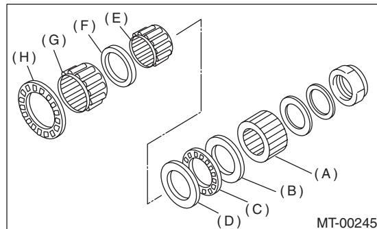
(A) Differential bevel gear sleeve
