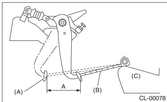
(A) Clutch pedal (Full stroke condition)
