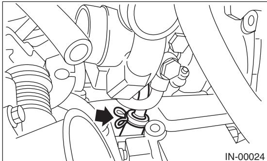
2) Install the turbocharger to intake duct.
