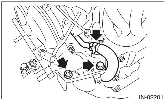
5) Install the joint pipe to turbocharger.
