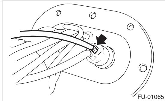
3) Remove the fuel temperature sensor (A).
