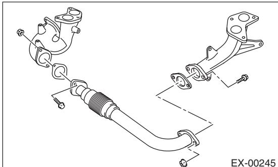
2) Install the front exhaust pipe cover.
