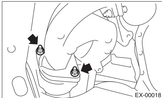
6) Install the exhaust manifold lower cover (RH) and the exhaust manifold cover (LH).
