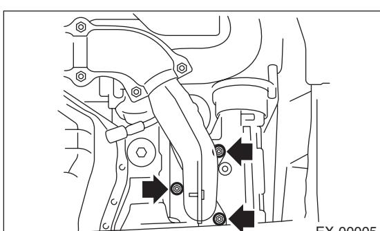
5) Connect the exhaust manifold (RH) to turbocharger joint pipe.
