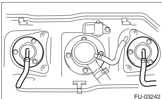
4) Remove the bolts which install the fuel cut valve.
