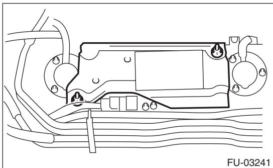
3) Move the clip and disconnect the evaporation hose from the fuel cut valve.
