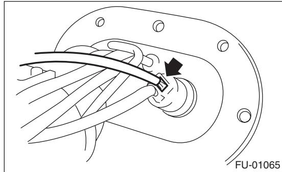
3) Remove the fuel temperature sensor (A).
