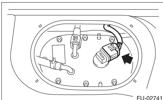
6) Disconnect the quick connector, then disconnect the fuel delivery hose. <Ref. to FU(H4SO)-60, REMOVAL, Fuel Delivery and Evaporation Lines.>
