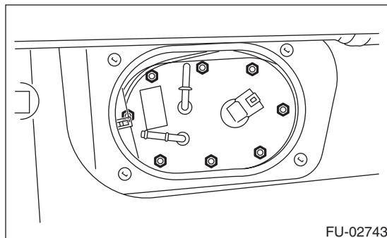
9) Remove the fuel pump assembly from the fuel tank.
