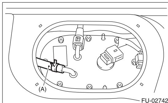
8) Remove the nuts which install fuel pump assembly onto fuel tank.
