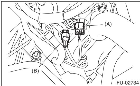
(A) Front oxygen (A/F) sensor connector
