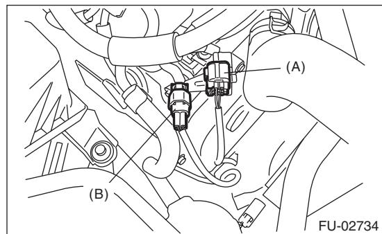
(A) Front oxygen (A/F) sensor connector
