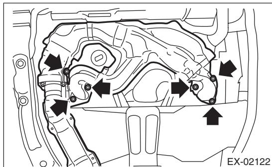
5) Tighten the bolt which holds the center exhaust pipe to exhaust pipe.
