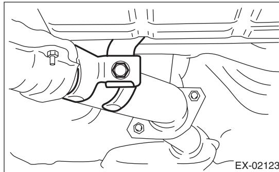
7) Tighten the nuts which hold front exhaust pipe to cylinder heads.
