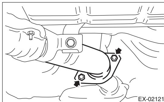
6) Tighten the bolt which holds center exhaust pipe to hanger bracket.
