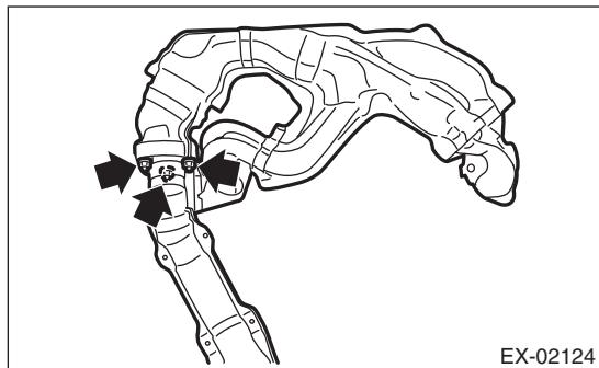
3) Install the front and center exhaust pipe assembly to the vehicle.
