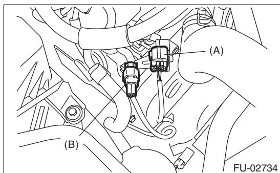
(A) Front oxygen (A/F) sensor connector
