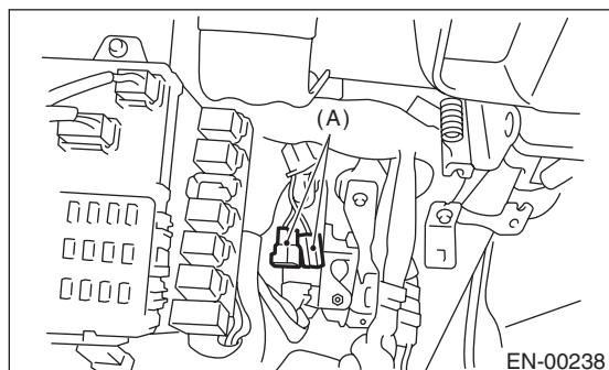
6) Connect the SDI to data link connector located in the lower portion of the instrument panel (on the driver's side).
