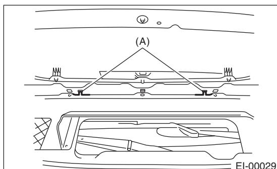
6) Install the front hood duct with the five screws and clip (A).
