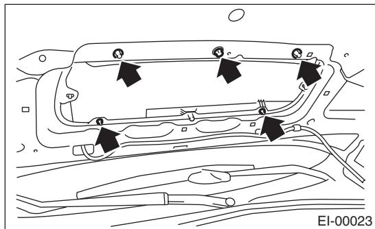
3) Remove three black clips and remove the front hood grille.
