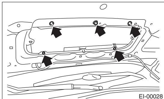
5) Hook the two hooks (A) of hood duct to the hood holes.
