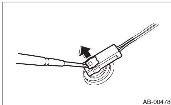
(2) Pull the connector to disconnect from driver's airbag module assembly or retractor assembly.
