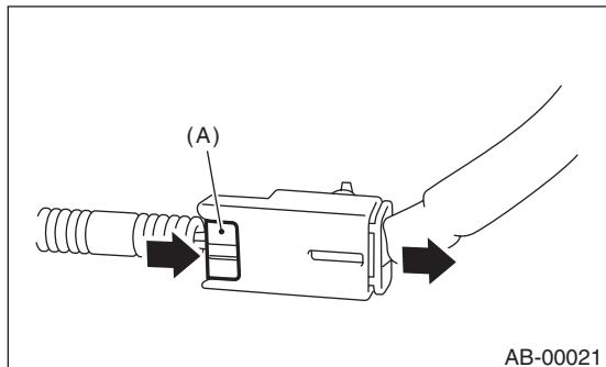
(2) With the slide lock pushed, pull it in the direction of arrow and disconnect the connector.
