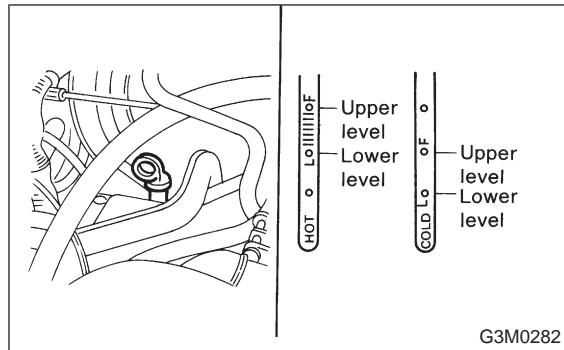
2) Make sure the vehicle is level. After selecting all positions (P, R, N, D, 3, 2, 1), set the selector lever in "P" range. Measure fluid level with the engine idling.
