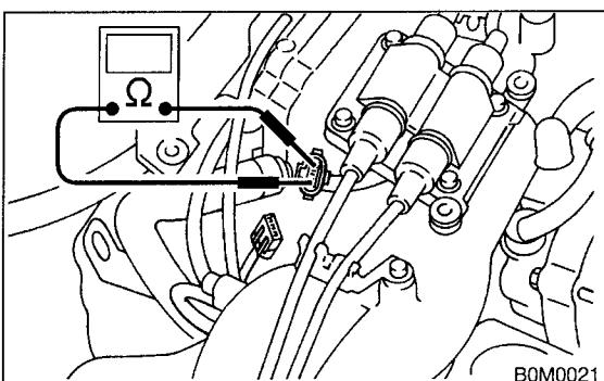
1) Check for open circuit. (range:  $\Omega \times 1K$ )
