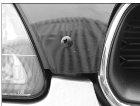
New installation with metal clip and screw
