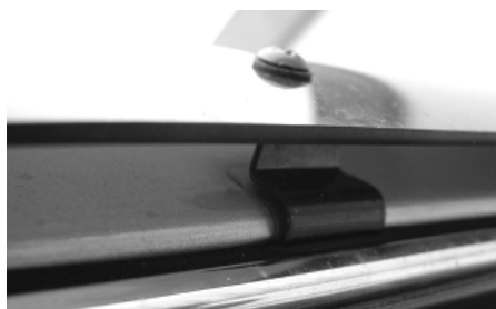
Installation of Center Clip on New Deflector requires R&R of Grille.
