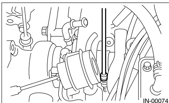
3) Install the oil pipe to turbocharger.
