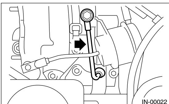
4) Install the joint pipe to turbocharger.
