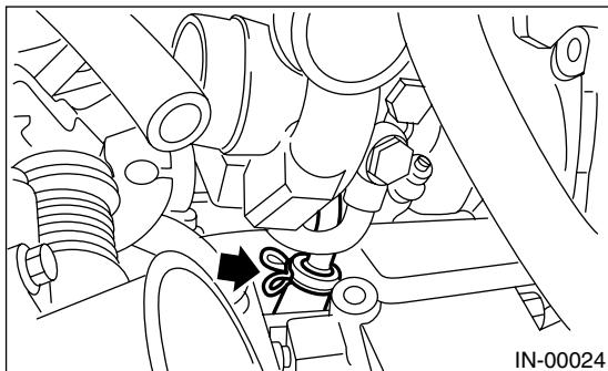
2) Install the turbocharger to intake duct.
