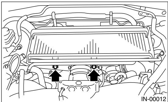
3) Disconnect hose from air bypass valve.
