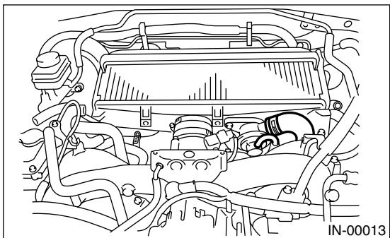
4) Remove bolt which secure intercooler to bracket.
