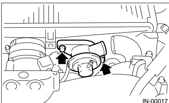
2) Remove intercooler duct from intercooler.
