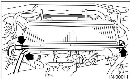
2) Remove PCV pipe from intercooler.
