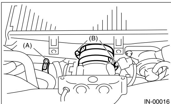
7) Disconnect intercooler duct from turbocharger.
