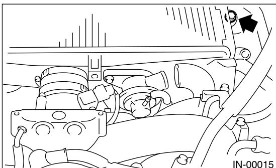
5) Loosen clamp (A) which connects turbocharger and intercooler duct.
