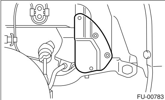
7) Apply SUBARU CRC or its equivalent to the threaded portion of front oxygen (A/F) sensor, and leave it for one minute or more.
