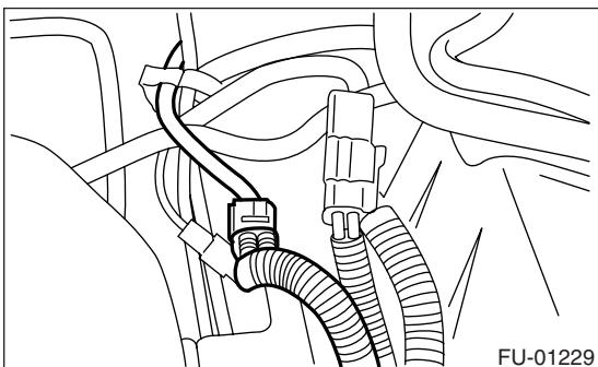
3) Disconnect the engine harness fixed by clip (A) from the bracket (B).
