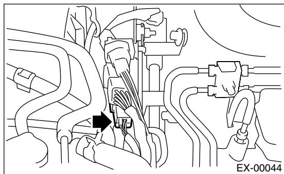
3) Remove the front oxygen (A/F) sensor. <Ref. to FU(H4DOTC)-37, REMOVAL, Front Oxygen (A/F) Sensor.>
