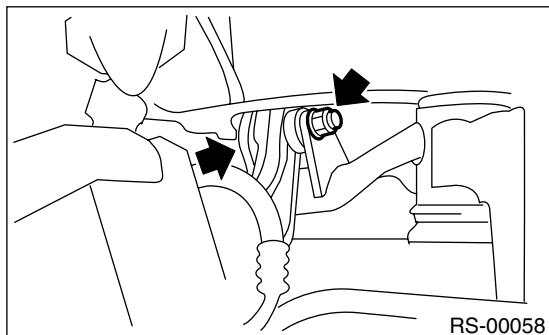
4) Remove bolts which secure link upper to rear arm and detach link upper.
