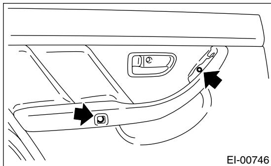
4) Remove seven clips (A) of trim panel using clip remover to remove trim panel.
