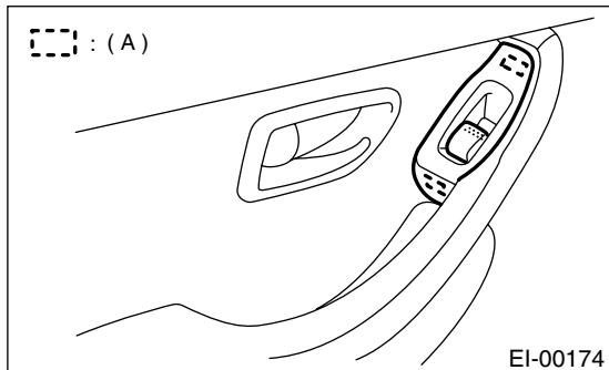
3) Remove two screws and clips.
