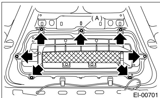
5) Install the hood insulator with new clips.
