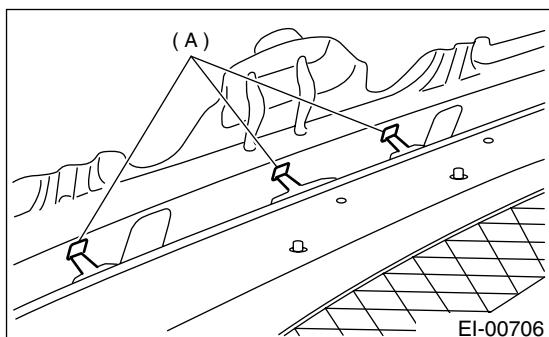
4) Install hood duct with clip (A) and seven bolts.
