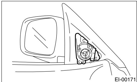
6) Remove seven clips (A) of trim panel using clip remover to remove trim panel.
