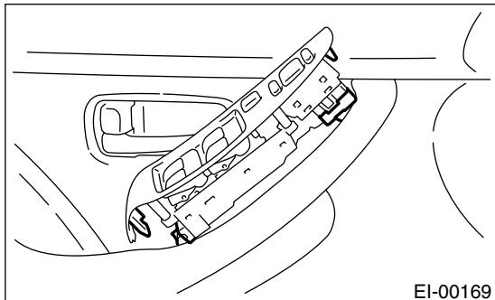
4) Remove three screws and clips.
