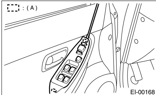
3) Disconnect electrical connectors from power window main switch and mirror switch.
