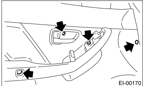
5) Remove gusset cover. Disconnect electrical connectors to remove speaker.
