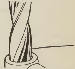
FIG. 16 Drill out the damaged threads with specified drill bit. Drill completely through the hole or to the bottom of a blind hole
