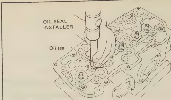
FIG. 61 Installing the valve oil seal with a driver
