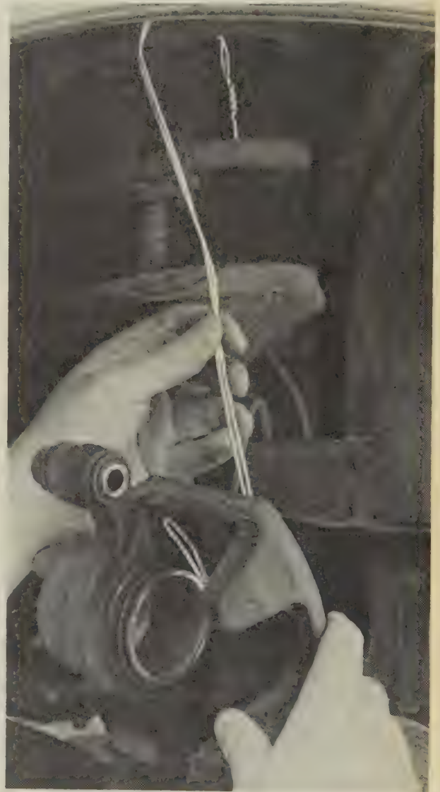
FIG. 23b Support the caliper from the strut spring using a piece of wire
