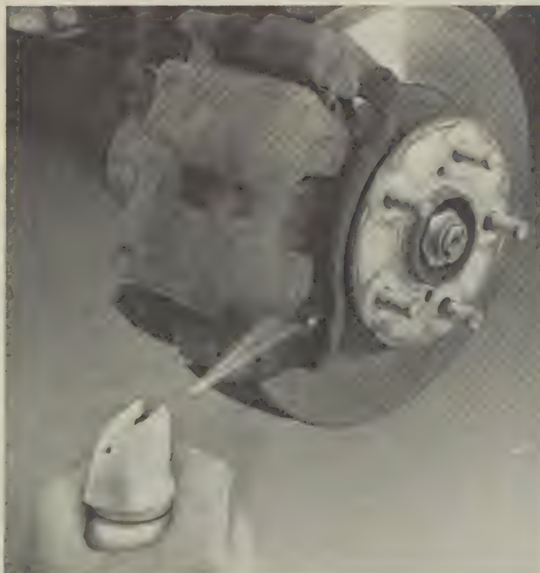
FIG. 21b Clean the brakes before disassembly, use a suitable brake cleaning agent
