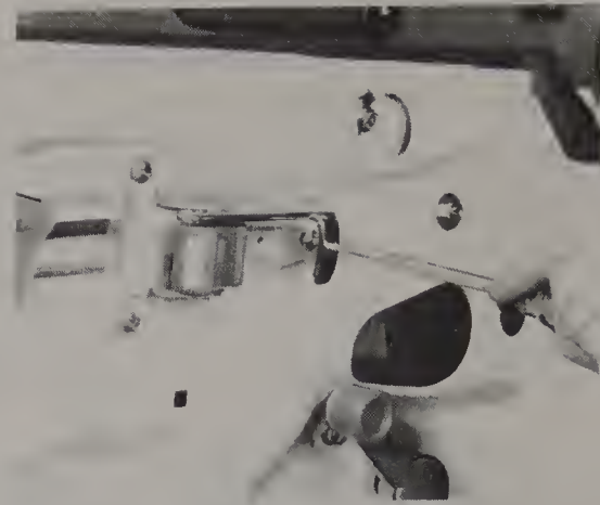
13.4 Removing the interior door handle mounting screws
