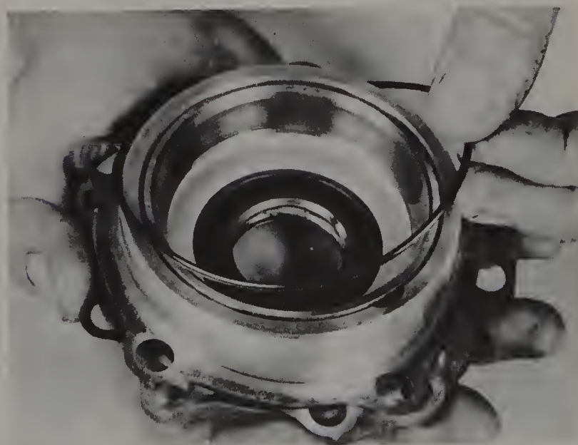
10.6 Replace the retainer O-ring with a new one
