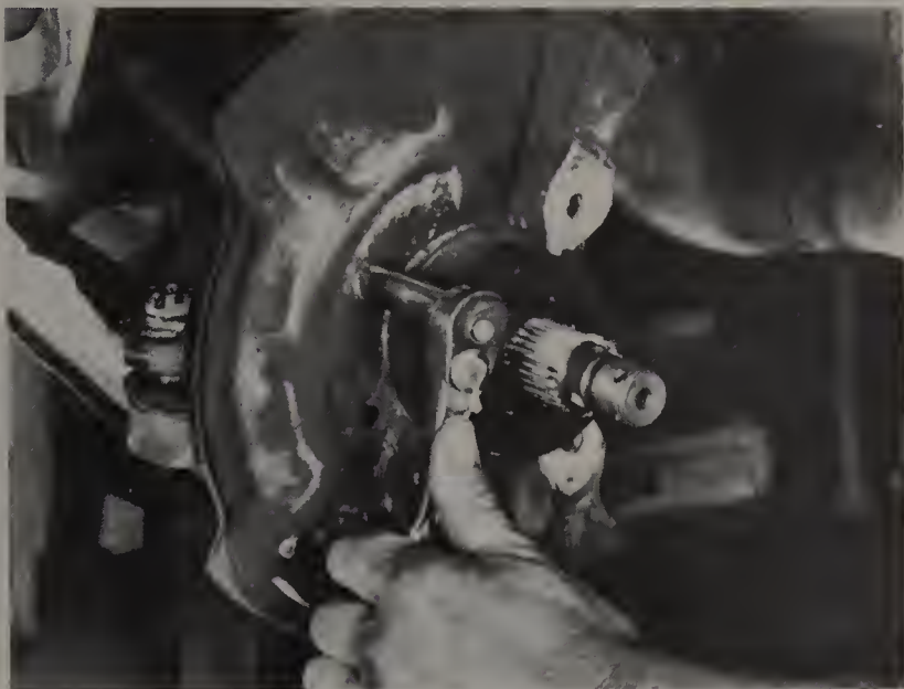
9.3 Remove the bolts holding the backing plate to the steering knuckle
