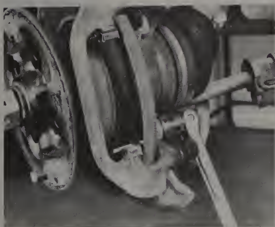
8.2 Remove the caliper support mounting bolts
