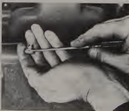
15.1B Position the screwdriver between the outside and inside lips and pry
