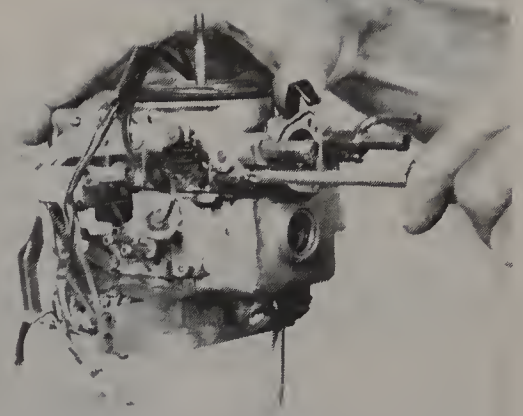
9.6A Remove the vent solenoid valve housing
