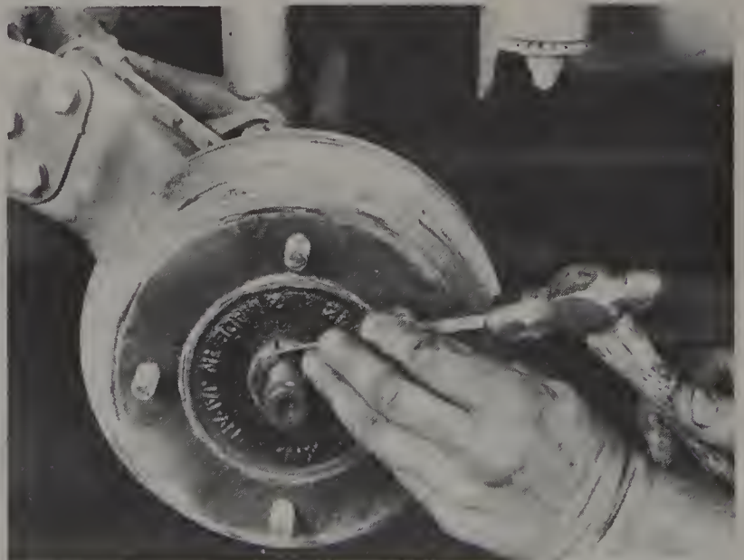
10.17 Loosen the conical spacer
