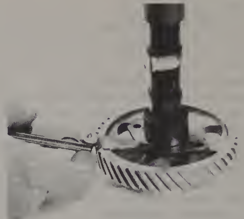
26.3 Measuring camshaft thrust clearance with a feeler gauge
