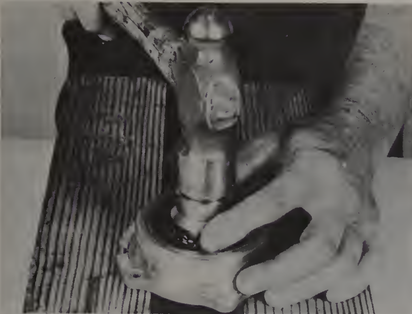
10.7 Use a socket to drive the old oil seal out of the retainer
