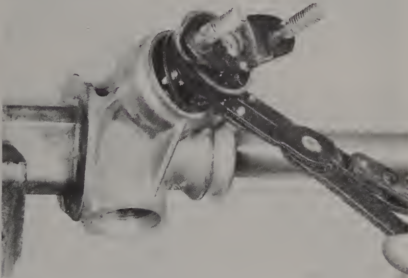
21.10 Remove the retaining ring from the pinion
