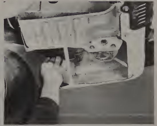
18.2B Remove the side bumper-to-vehicle body bolts
