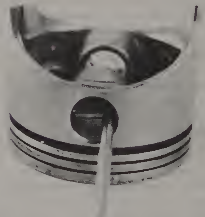
27.12B A telescoping gauge is used to determine the piston pin bore size
