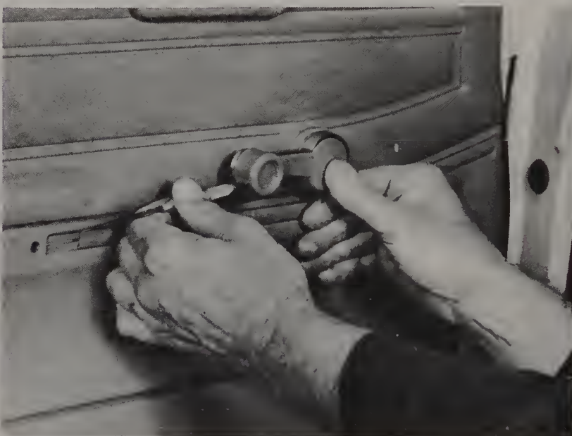
12.2 Removing the window regulator handle clip
