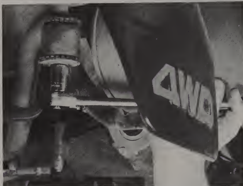
12.7 Remove the rear bracket assembly mounting nuts
