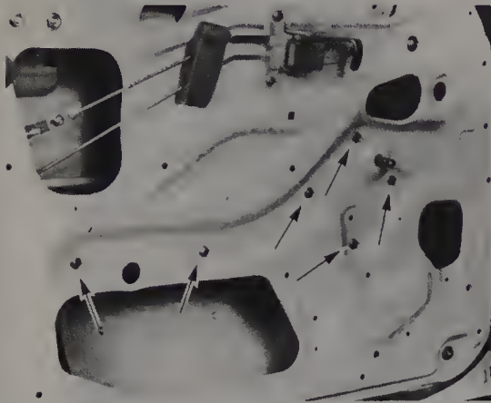
13.19 Detach the regulator by removing the regulator baseplate bolts and the regulator channel bolts (arrows)
