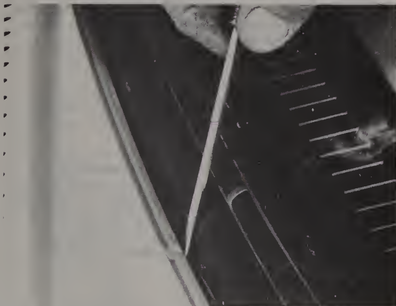
27.5 Carefully maneuver the rubber lip to the underside of the cowl with a screwdriver
