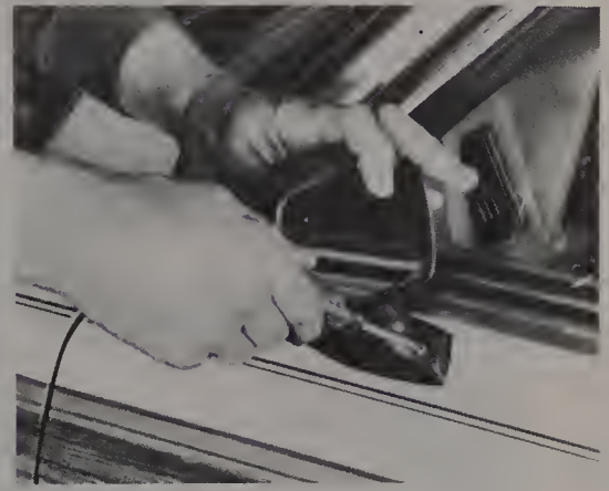
13.22 Removing the rear view mirror mounting screws
