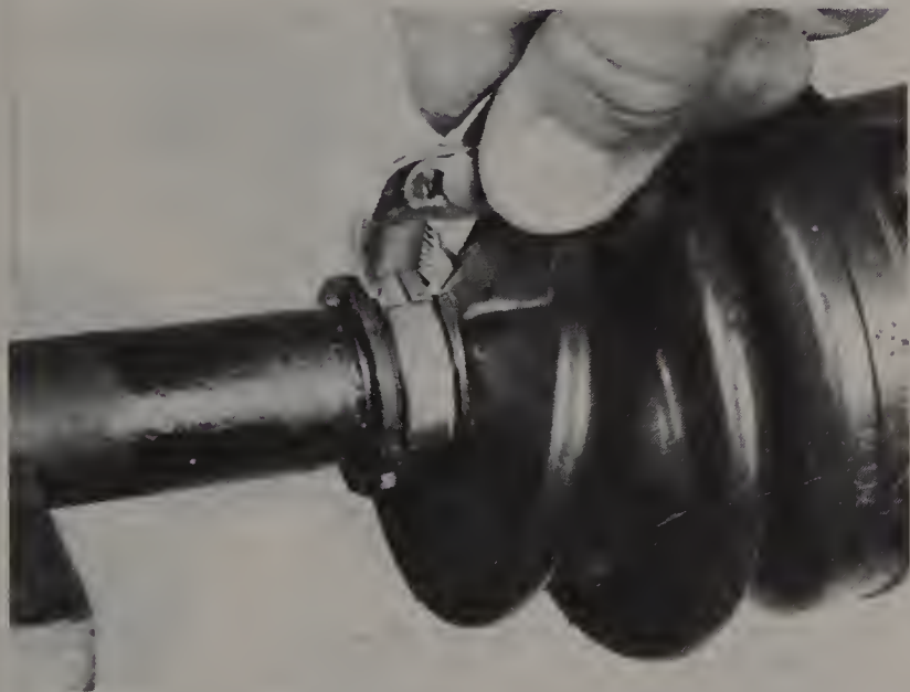
8.11 Cut off the excess metal band, fold under the locking tabs and bend the locking tabs into position
