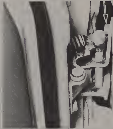
14.8 Adjustments to the door are made with the hinge body mounting bolts (arrow)
