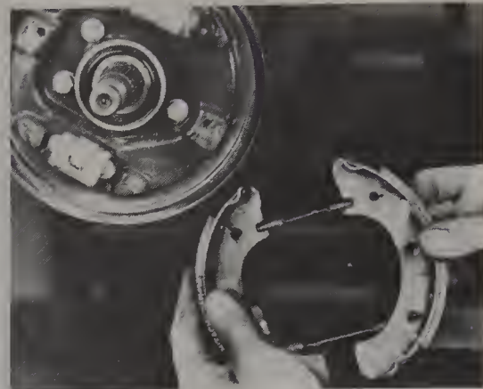
11.6 Remove the shoes with the springs
