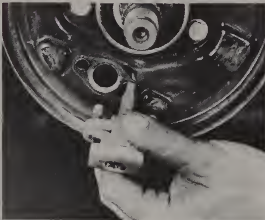
12.2 Remove the adjuster from the brake backing plate
