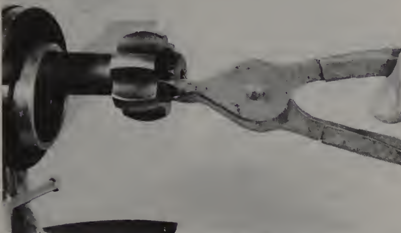
9.9 Remove the retaining ring from the end of the axleshaft
