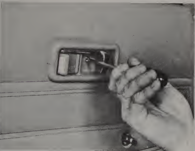
12.3 Removing the interior door handle cover screw
