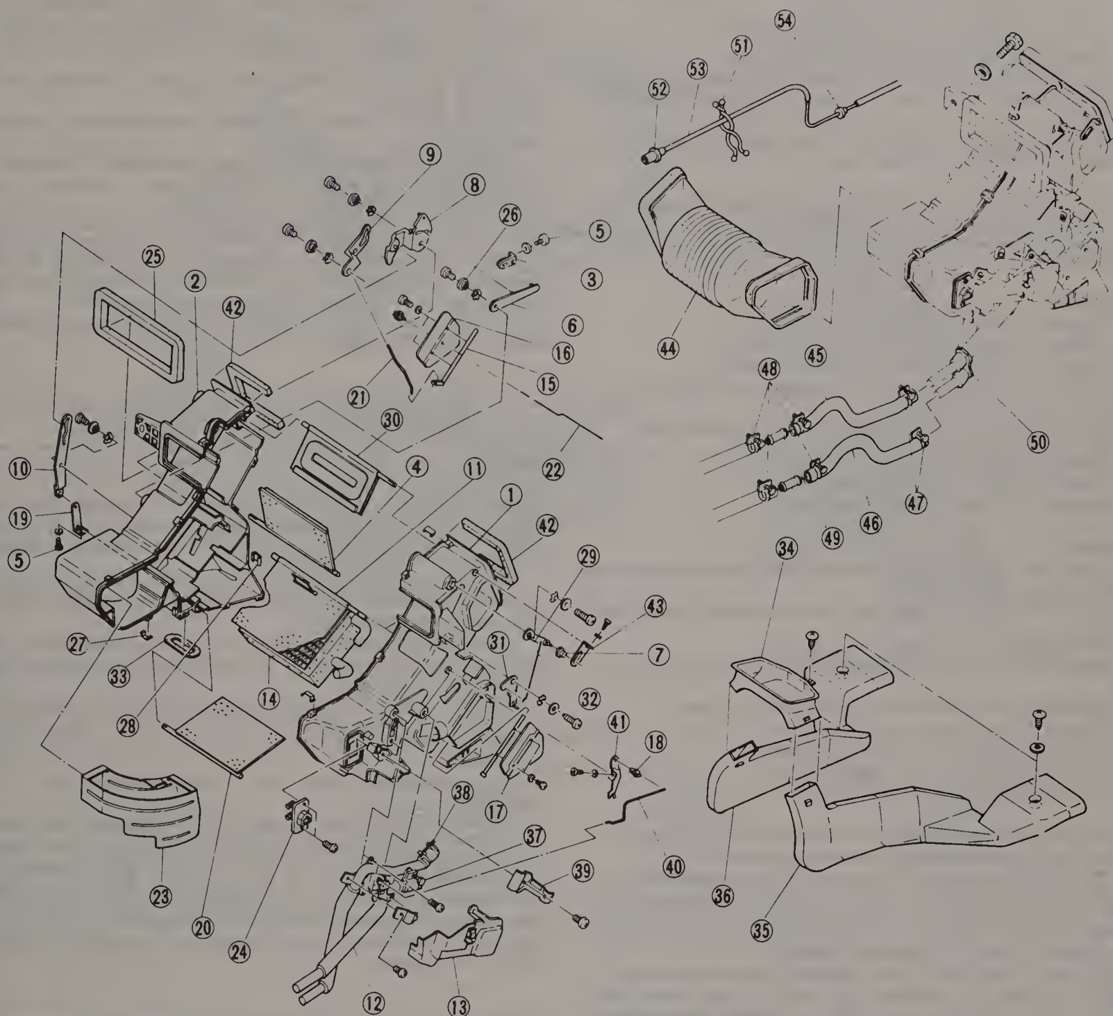
Fig. 3.12 Heater unit and duct components – exploded view (Sec 8)
