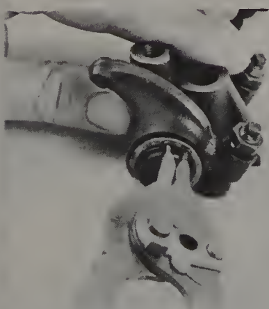
11.3 Removing the snap-ring from the rocker arm shaft
