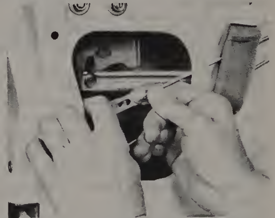
13.44 Connect the upper linkage to the latch linkage and install the screw (do not tighten it at this time)
