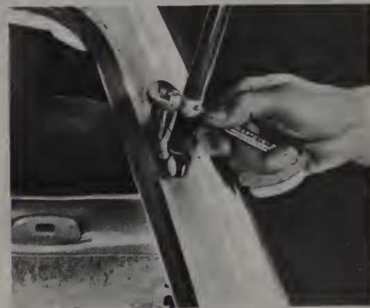
16.7B ... and then the bottom stay mounting bolts
