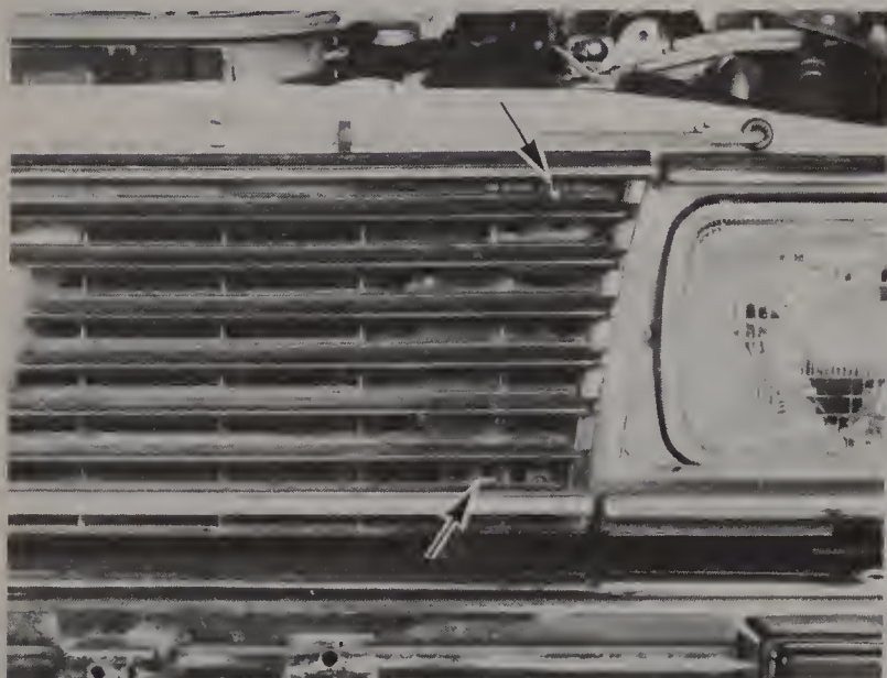
17.2 Remove the grille mounting screws (arrows)
