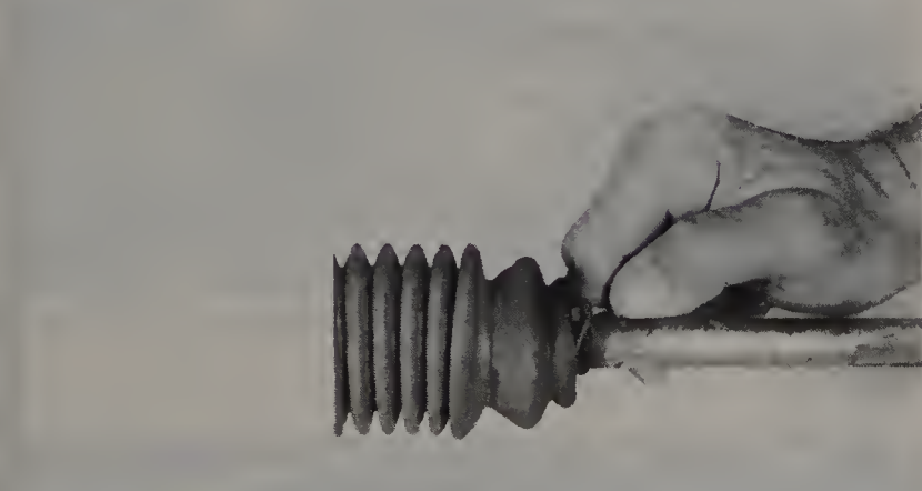
18.8 Remove the small boot retaining spring
