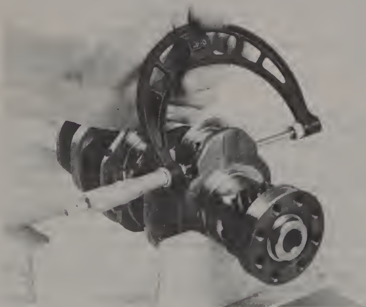
25.3 Measuring a connecting rod journal diameter with a micrometer
