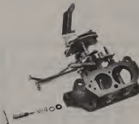
9.36 The throttle chamber with the idle mixture screw and lock pin
