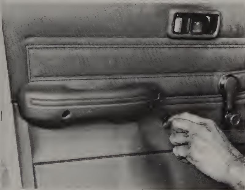
12.1 Removing the door armrest screws
