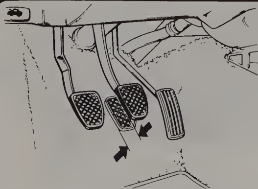
Fig. 1.22 Checking brake pedal free play (Sec 28)
