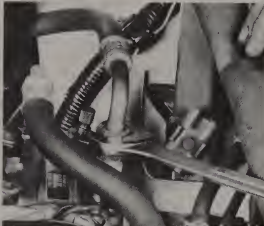
4.14 Separate the hoses from the air conditioning compressor only after you have had the system evacuated
