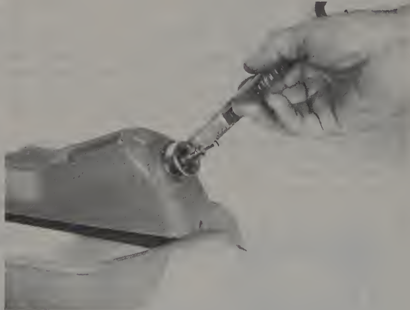
9.11 Remove the nut holding the lighting switch to the panel
