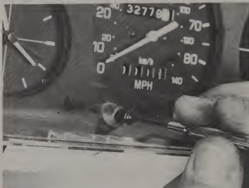
6.8 Remove the adjustment knobs to gain access to the meter interior
