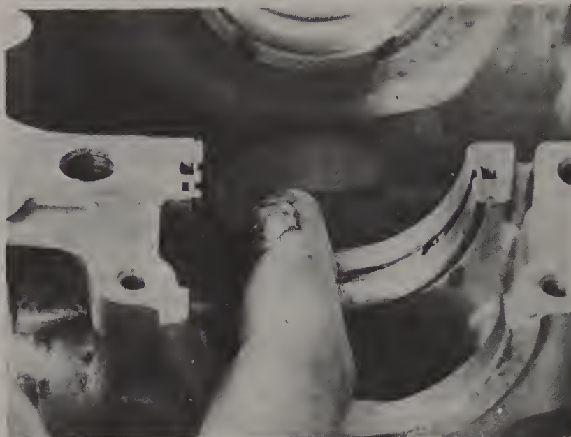
29.12 Apply engine assembly lube to the main bearings before installing the crankshaft
