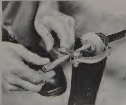
14.6 Remove the torsion bar from the outer arm with a puller
