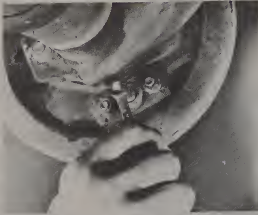
11.4 Back-off the adjuster screw completely
