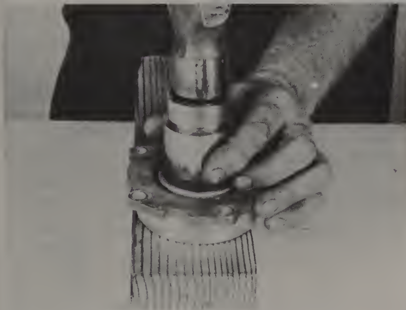
10.8 Carefully install the new seal flush with the retainer
