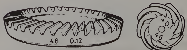
Fig. 7.20 Drive pinion and crown gear match mark locations (Sec 9)
