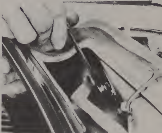
14.6 Remove the retaining nut from the wiper arm linkage connected to the wiper motor
