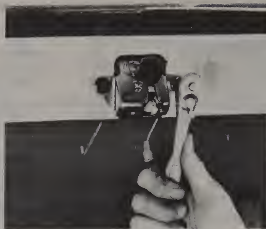
15.5 Remove the latch from the rear gate
