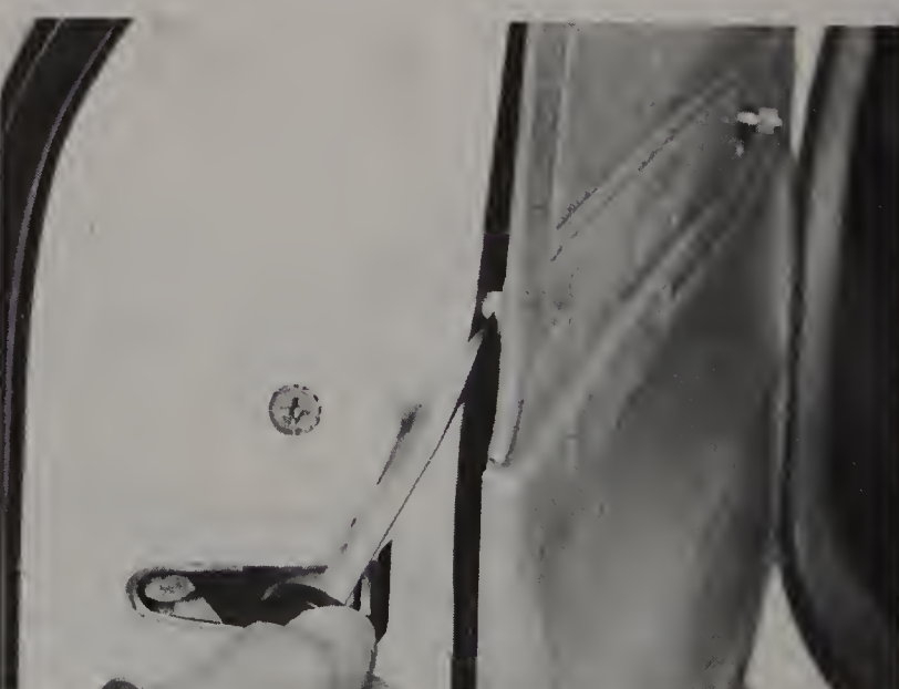
12.4 Carefully pry the door panels away from the door to remove them
