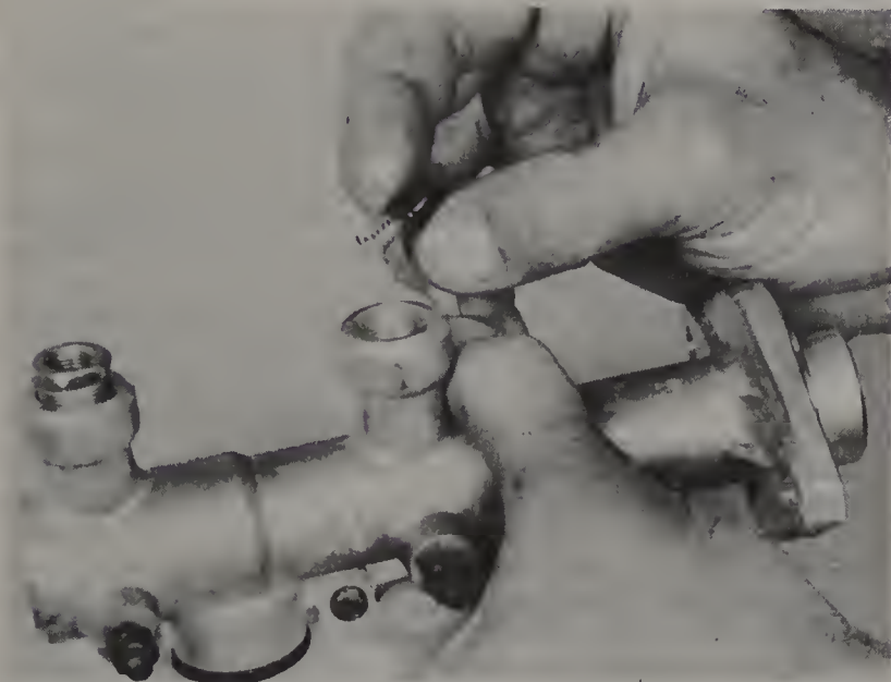
16.8 Install the check valve and spring
