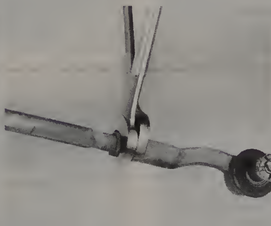
18.6 Loosen and back the jam nut away from the tie-rod end
