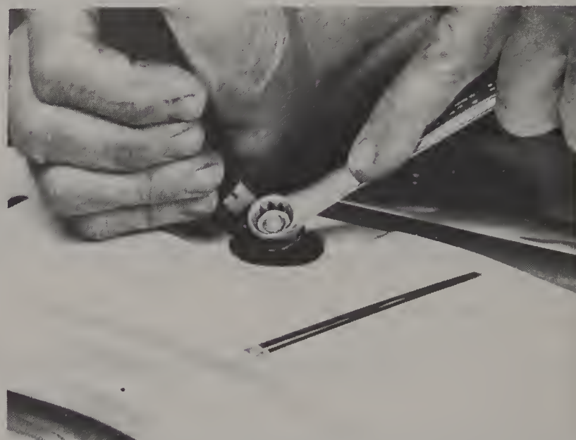
13.2 Remove the wiper arm mounting nut
