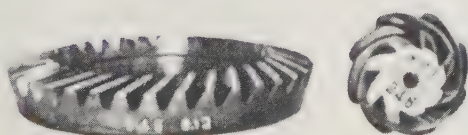
Fig. 6.22. Crown gear and drive pinion match marks
