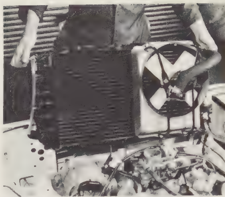
5.9 Removing the radiator
