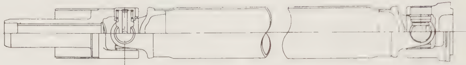
Fig. 7.13. Propeller shaft (4WD)
