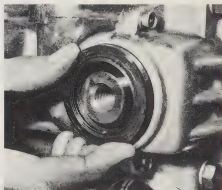
22.25 ... and then the crankshaft oil seal
