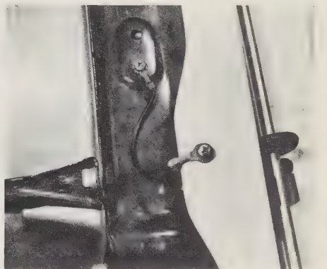
5.9b Disconnect the ground lead from the top of the radiator and ...
