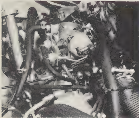
5.5 Disconnect the fuel delivery hose
