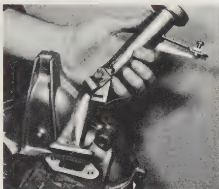
22.22 Fitting the oil filler duct on the crankcase
