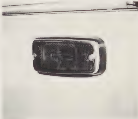
30.1 Remove the lens securing screws, take off the lens
