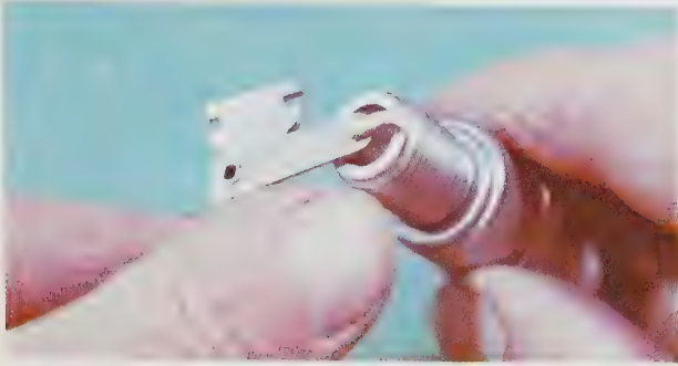
Measuring plug gap. A feeler gauge of the correct size (see ignition system specifications) should have a slight 'drag' when slid between the electrodes. Adjust gap if necessary
