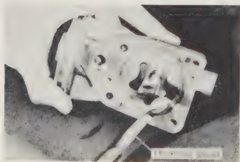
Fig. 1.28. Measuring the clearance between the pump body and rotor
