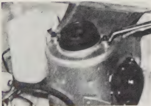
Fig. 11.22. Removing the damper strut upper attaching nuts (Sec. 11)
