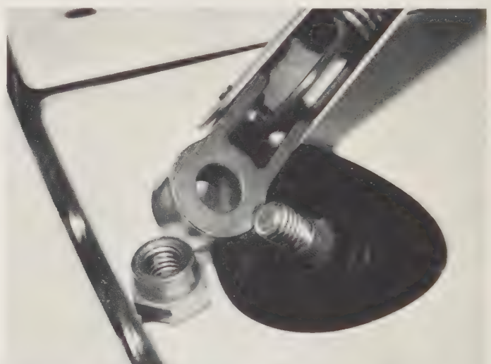
16.2b ... and lift the wiper arm off
