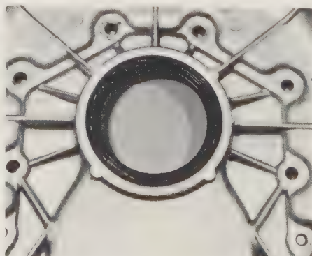
22.17a Press oil seal into the flywheel housing ...
