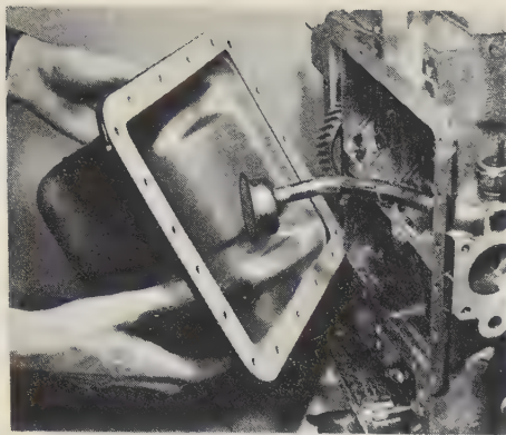
22.18 Fitting the crankcase oil pan
