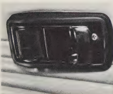
10.3a Remove the cover retaining screw ...
