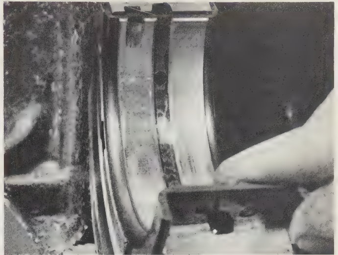
22.2 Fit the crankshaft bearing shells in the casing
