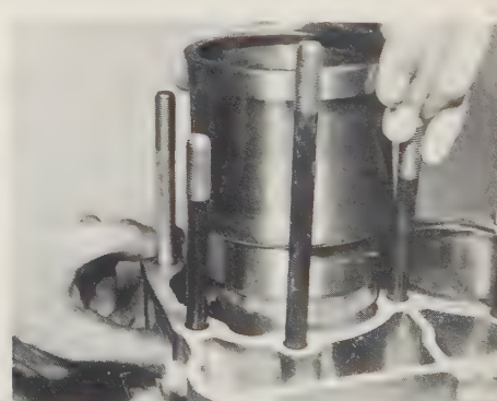
10.13b Lifting out the cylinder liner
