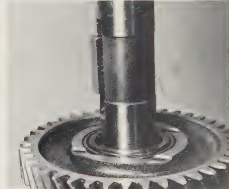
12.4b Insert the key in the drive pinion groove
