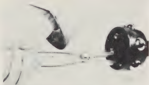
Fig. 7.8. Removing the snap-ring which retains the inner race
