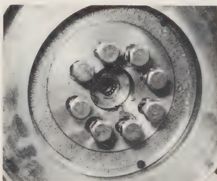
10.6a Remove the flywheel securing bolts ...
