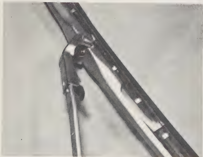
16.4a Remove the wiper arm blade by depressing the retaining spring ...
