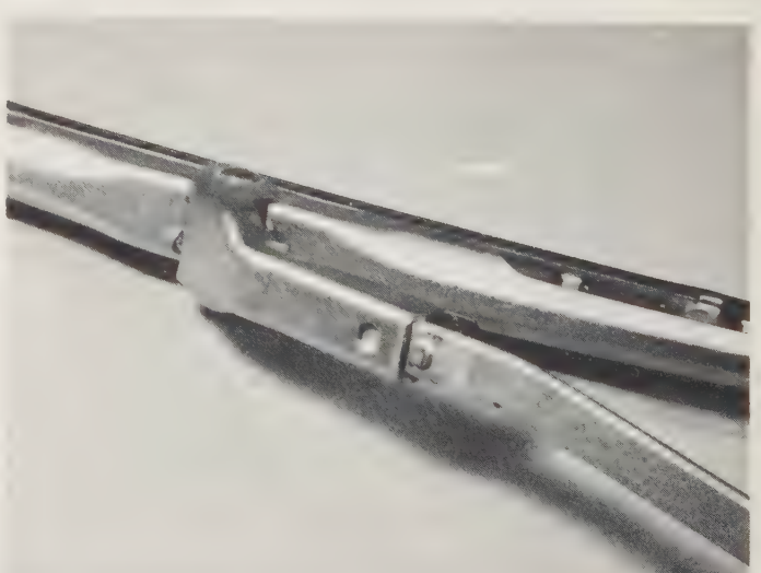
16.4b ... and then pull the blade out
