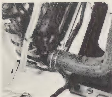
5.7 Disconnect the bottom radiator hose
