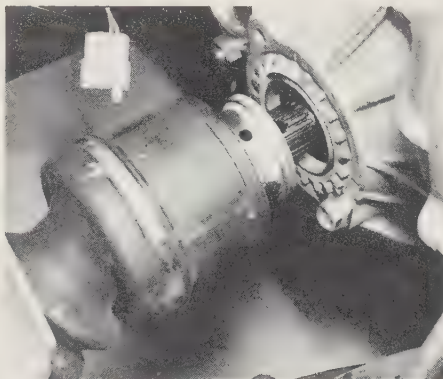
6.15 Pull the axle shaft off the transmission output shaft
