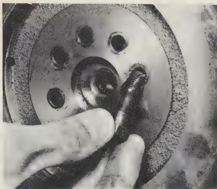
22.19a Fit the flywheel securing bolts
