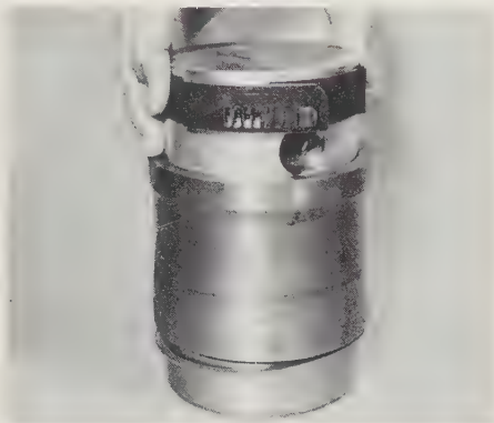
22.10a Compress the piston rings with a piston ring band and fit the piston in the cylinder liner
