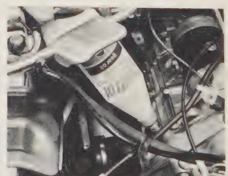
25.8b Replenish the transmission with hypoid gear oil
