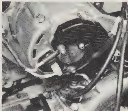
5.8a Disconnect the alternator leads
