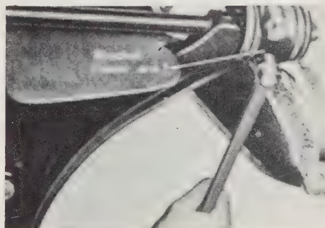
Fig. 11.15. Removal of lower arm bracket (FF - 1 model)
