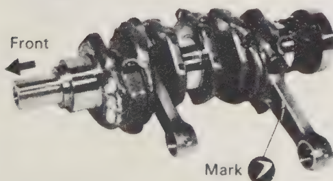
Fig. 1.30. Fitting direction of connecting rod
