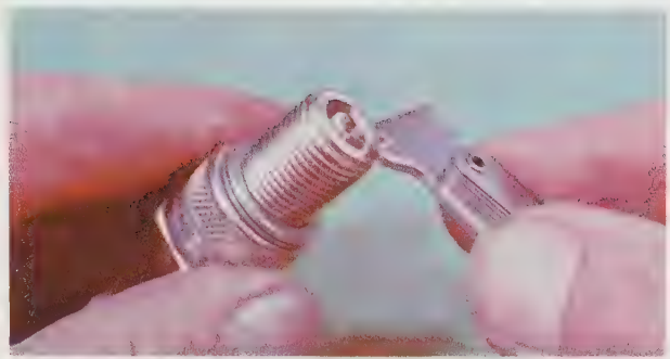
Adjusting plug gap. The plug gap is adjusted by bending the earth electrode inwards, or outwards, as necessary until the correct clearance is obtained. Note the use of the correct tool
