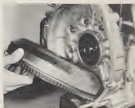
10.6b ... and lift off the flywheel
