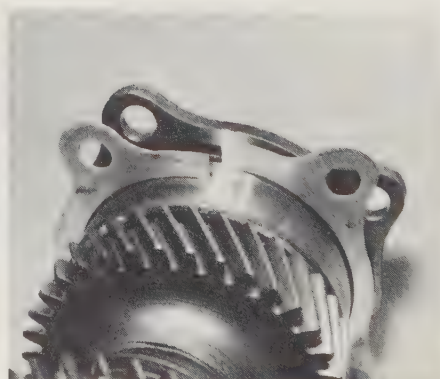
15.9a Fitting the shims on the drive pinion
