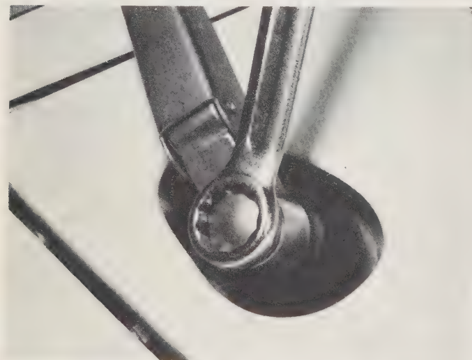
16.2a Remove the windshield wiper arm securing nut ...
