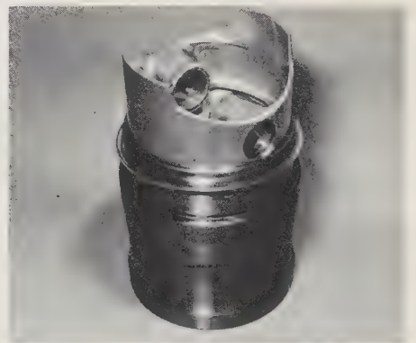
22.10b Position the piston in the liner
