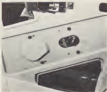
12.2 Remove the window regulator winding mechanism securing bolts
