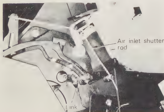
Fig. 2.15. Connecting the heater air inlet shutter rod
