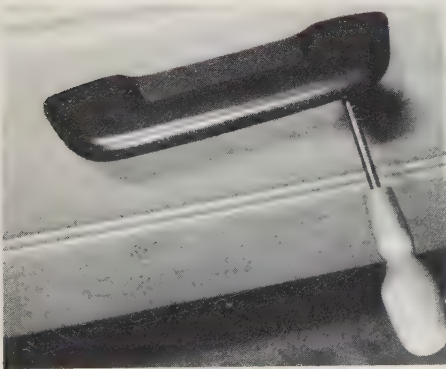
10.1 Removing the armrest attaching screws
