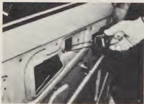
Fig. 12.12. Remove the interior door handle remote assembly
