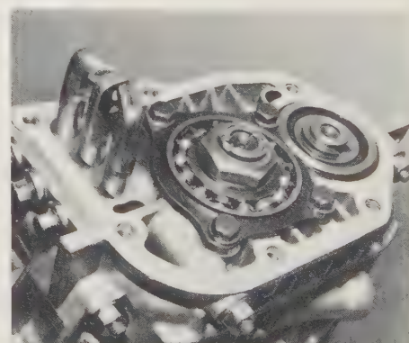
15.23b Shift rails in position for fitting the transmission cover
