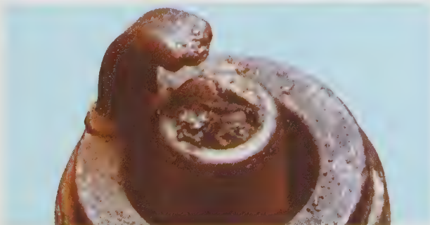
Electrode damage. Electrodes burned away; core nose has burned, glazed appearance. Fault: initial pre-ignition. Check: as for 'Overheating' but may be more severe. Discard plugs and remedy fault before piston or valve damage occurs
