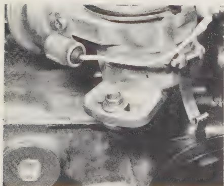
5.4 Remove the distributor retaining bolt
