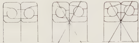
Fig. 11.9. Assemble the two halves of the bearing correctly (FF - 1)
