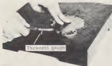
Fig. 2.10. Checking the water pump plate for warp
