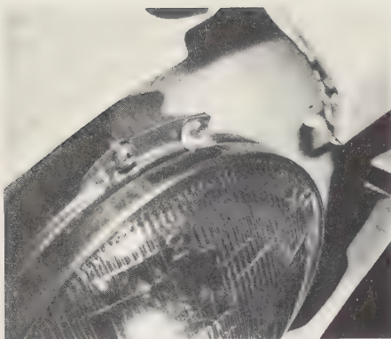
27.2a Remove the headlamp retaining screws ...
