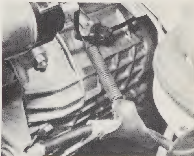
2.4 Remove the spring support from the clutch cable
