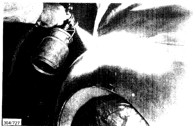
Applying etch primer to the bare metal surface.
