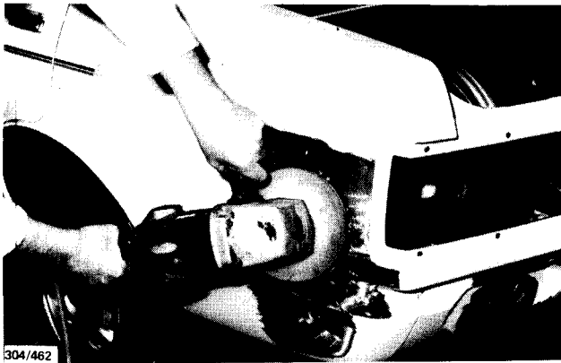
Removing the old paint finish from the damaged area using a disc sander.
