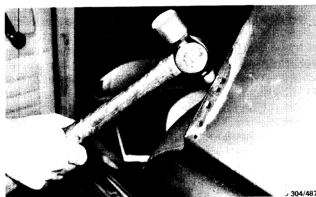
Using a ball peen hammer to tap down the rust affected area.
