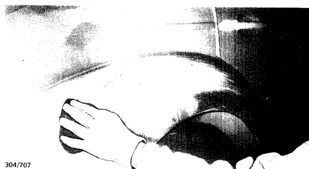
Removing any remaining paint or primer surfacer using steel wool soaked in stripper.
