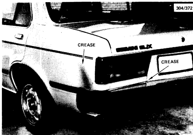
View of vehicle showing extent of panel damage prior to commencing repair operations.
