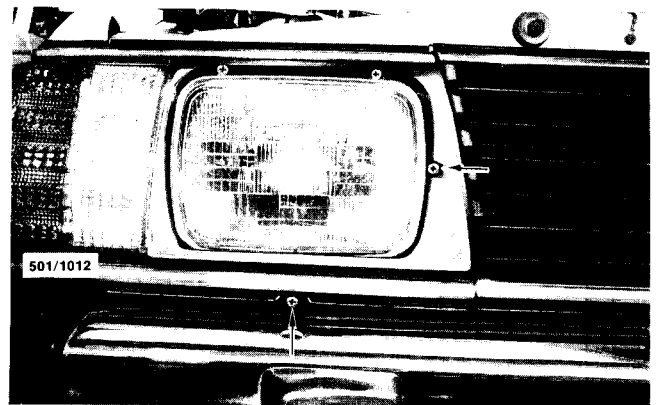
View showing the headlamp adjusting screws, 1981 model shown.
