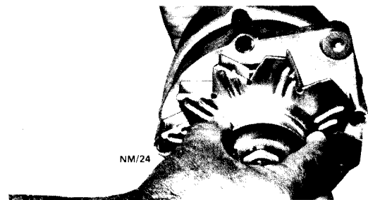
Spin the alternator pulley over by hand to check bearings for noise.
