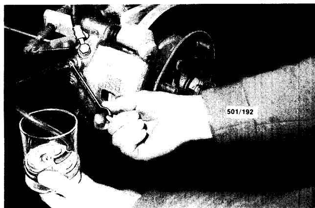
Method of bleeding air from the hydraulic brake system.
