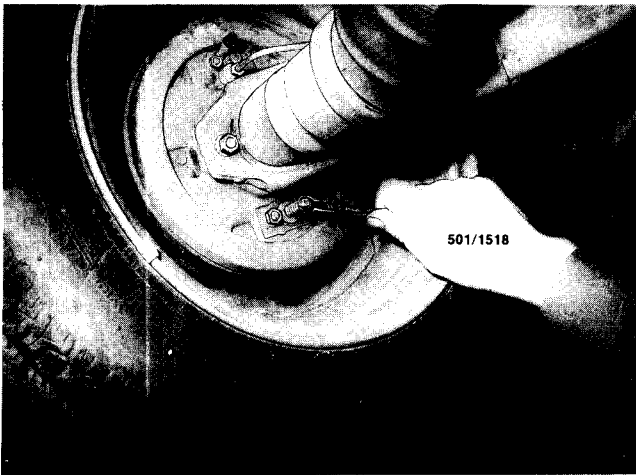
Method of adjusting the rear brakes, 1983 model shown.
