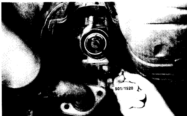
Using a suitable screwdriver, prise the oil seal from the rear of the transaxle rear extension.
