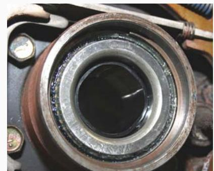
➤ If the snap ring doesn't properly engage the groove, the bearing isn't fully seated.
