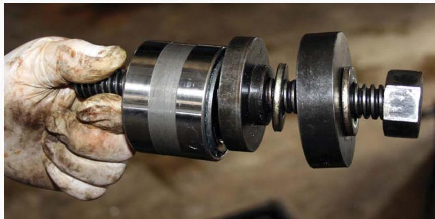
9 Screw the installation bolt through the housing and into the nut on the back of the housing. Secure the nut with a wrench and begin tightening the bolt with an air wrench and socket to seat the bearing.
