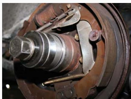
➤ Tools positioned to install the bearing.
