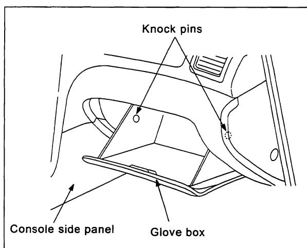
(3) Reinstall the glove box assembly as follows.
