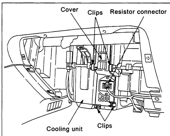
(2) Reinstall the cover, secure it using the clips and reconnect the resistor connector.
