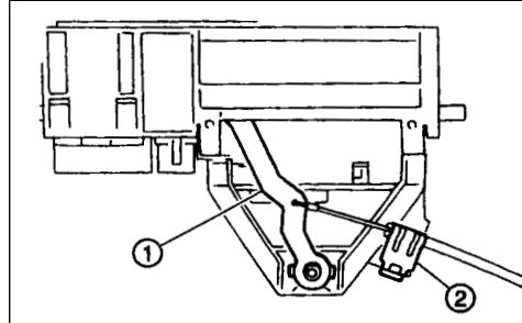
A misadjusted cable could allow heated air to mix with the cooler air and significantly increase the temperature of the air at the ducts. It is important that the air mix door be completely closed when in the A/C mode.
