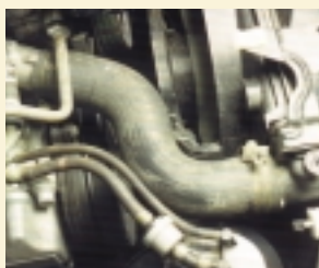
Cooling System Hoses
