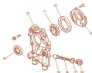
If you encounter a 2.5 liter DOHC Subaru engine with a leaking or dislodged front crankshaft oil seal, consider the oil pump as a possible cause. It may be necessary to remove the oil pump and examine the oil pump rear sealing plate before installing a new seal. The screws holding the rear sealing plate may be loose (by as much as 1/16-inch in some reported cases).
