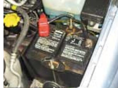
A battery that is below 11.6 volts can also be hydrated. This means there is lead sulfate in the separator that will form lead shorts once the battery charges. Because of these shorts, the battery may self discharge once the battery has been recharged.
