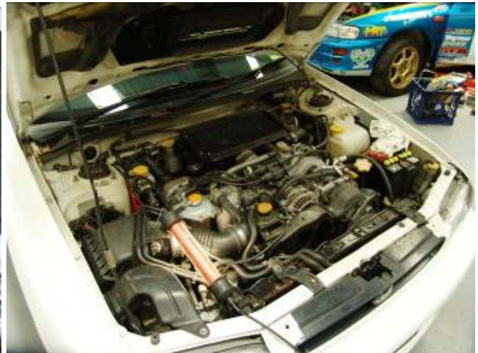
Standard engine bay, note revised inlet under inlet manifold
