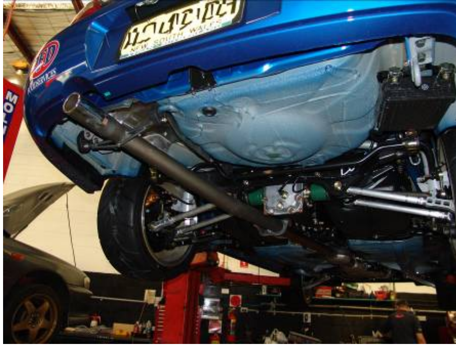
Version VIII STi Rear Suspension (Tarmac Rally car)
