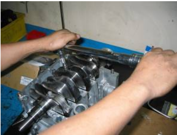
Torquing Rod Bolts for Clearance Check
