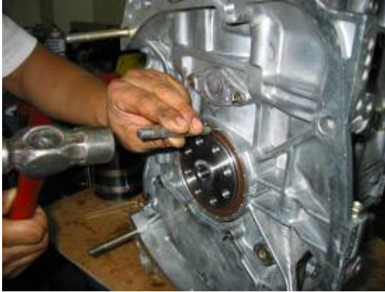
Staking Rear Main Oil Seal
