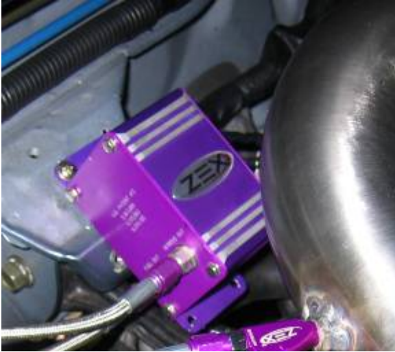
Pic Nitrous and Fuel Solenoid Box
