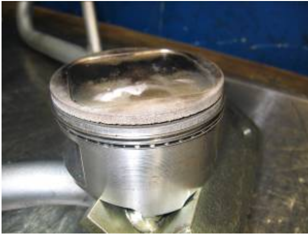
Long Term Detonation Damage
