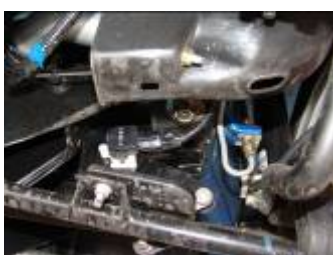
HID level sensor
