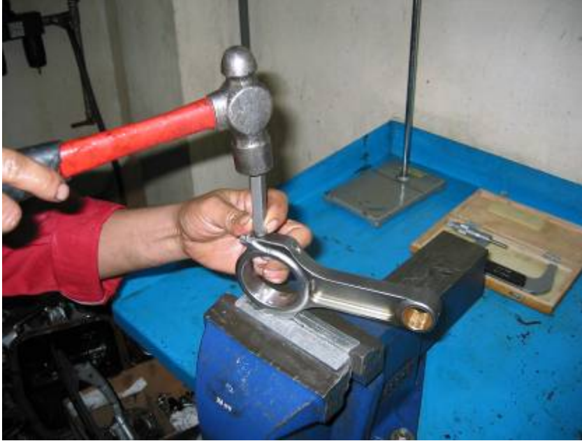
Marking Conrod to Cylinder Numbers
