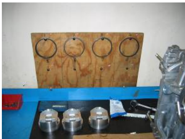
Piston Rings Ready for Fitting
