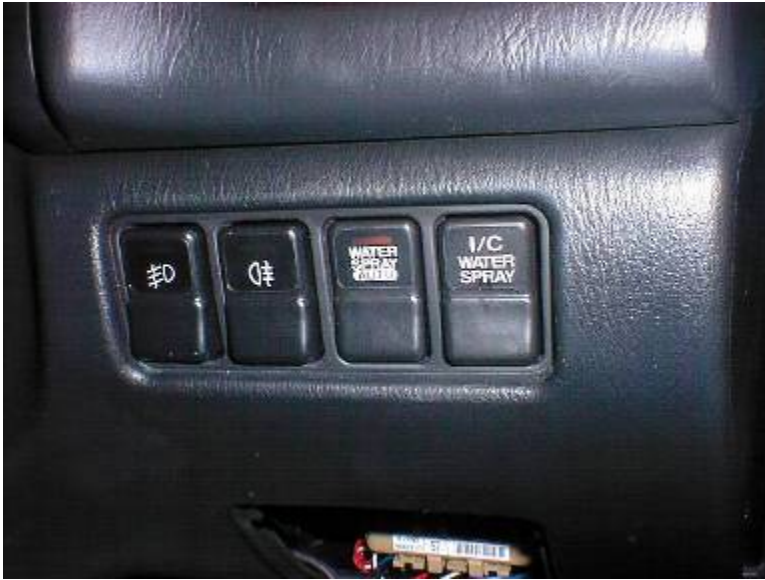
Factory switches for waterspray, "Auto" and "Manual"
