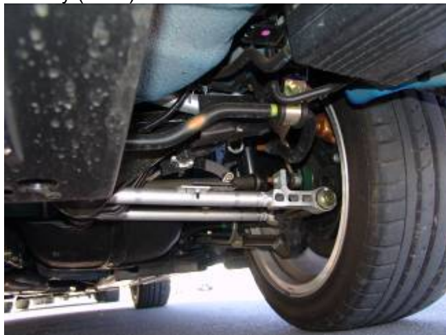
Rear suspension note sensor for HID lights
