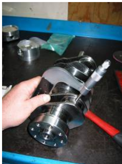
Measuring Crank Big End Journal Diameter
