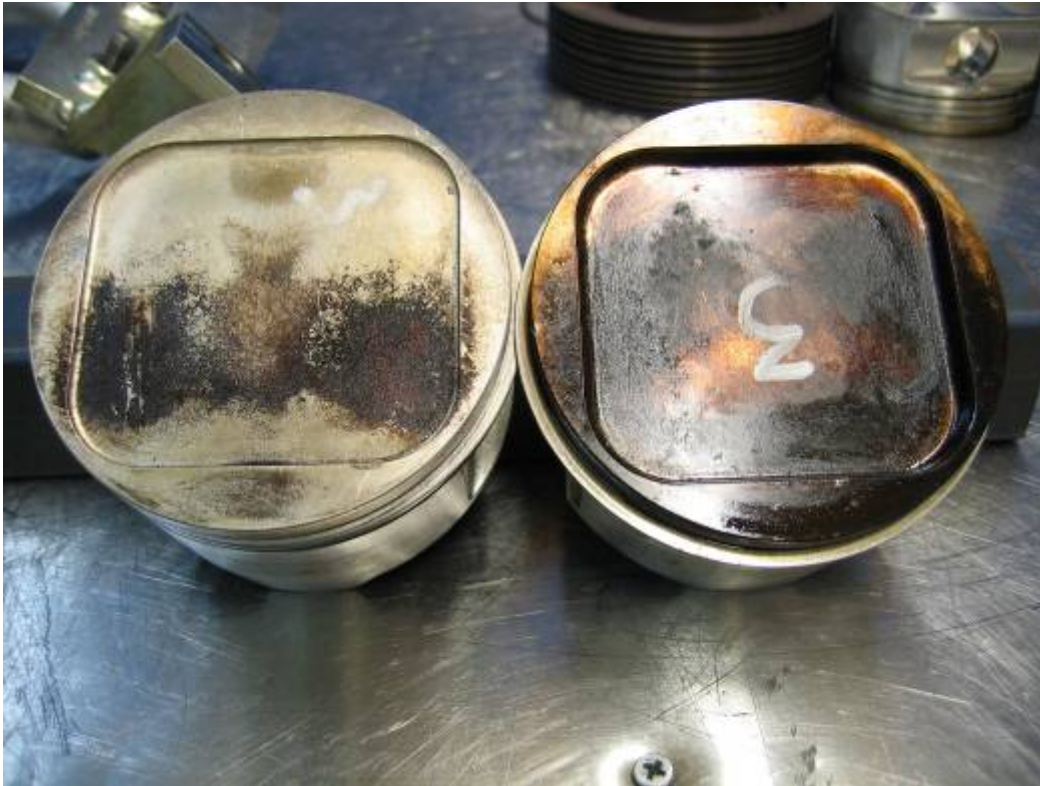
Note Detonation has Cleaned Carbon from Piston on Left Compared to Piston on Right
