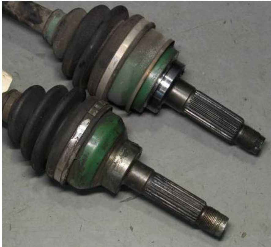
OE R160 Driveshaft vs R180
