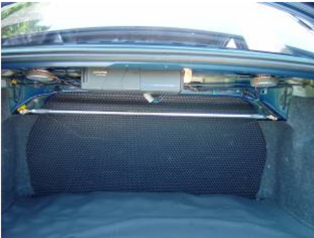
Rear Strut Brace
