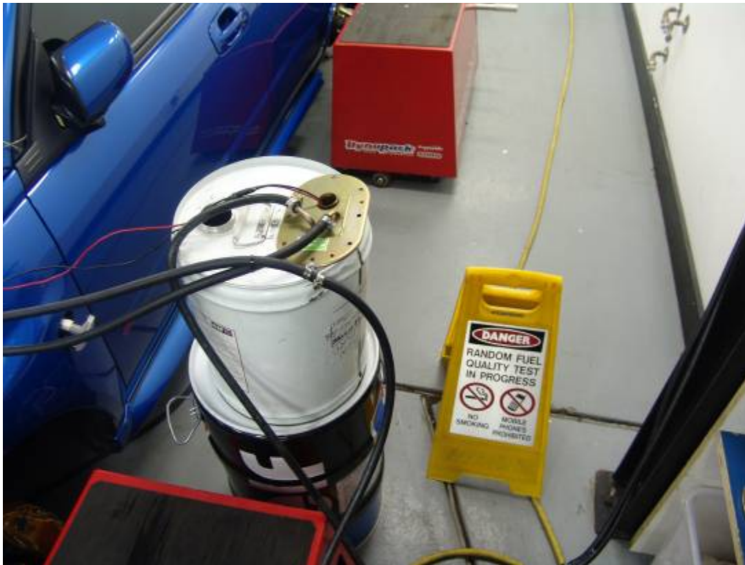
External Fuel Tank Test Rig
