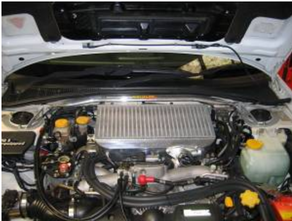
Pic Front Strut Brace
