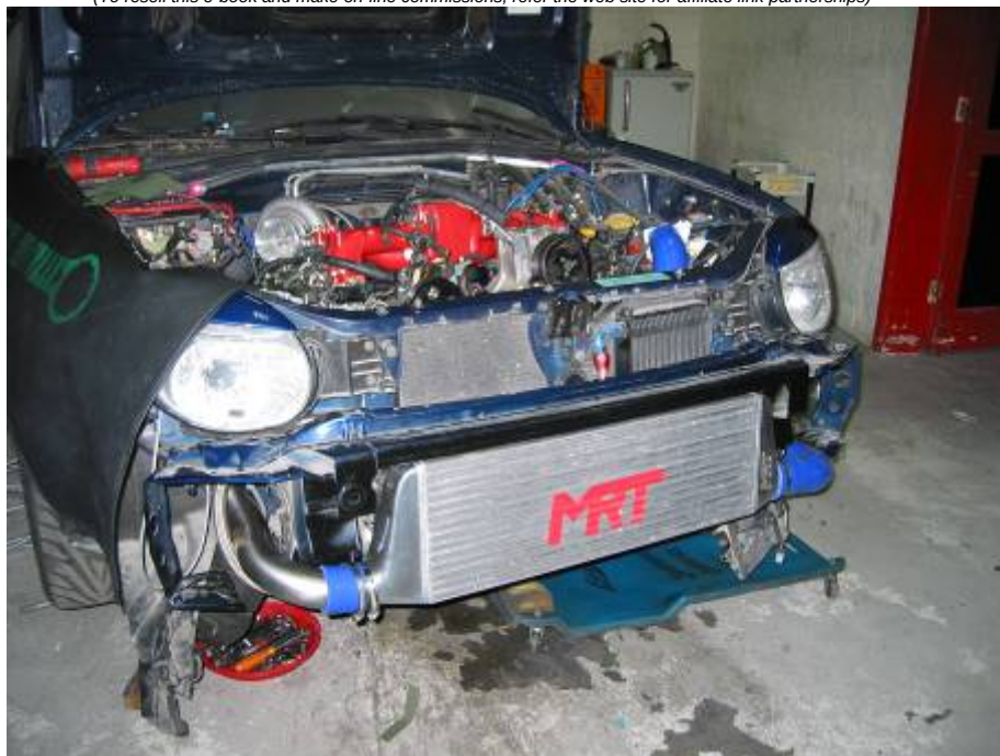
Angle Mounted Turbocharger Installed
