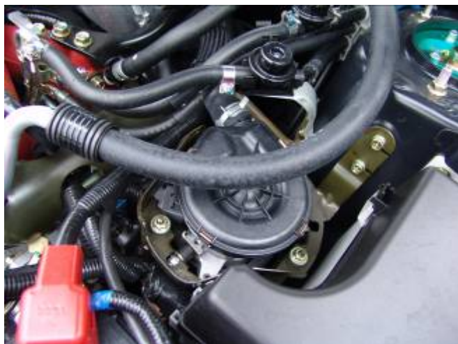
Air injection pump was new to this model
