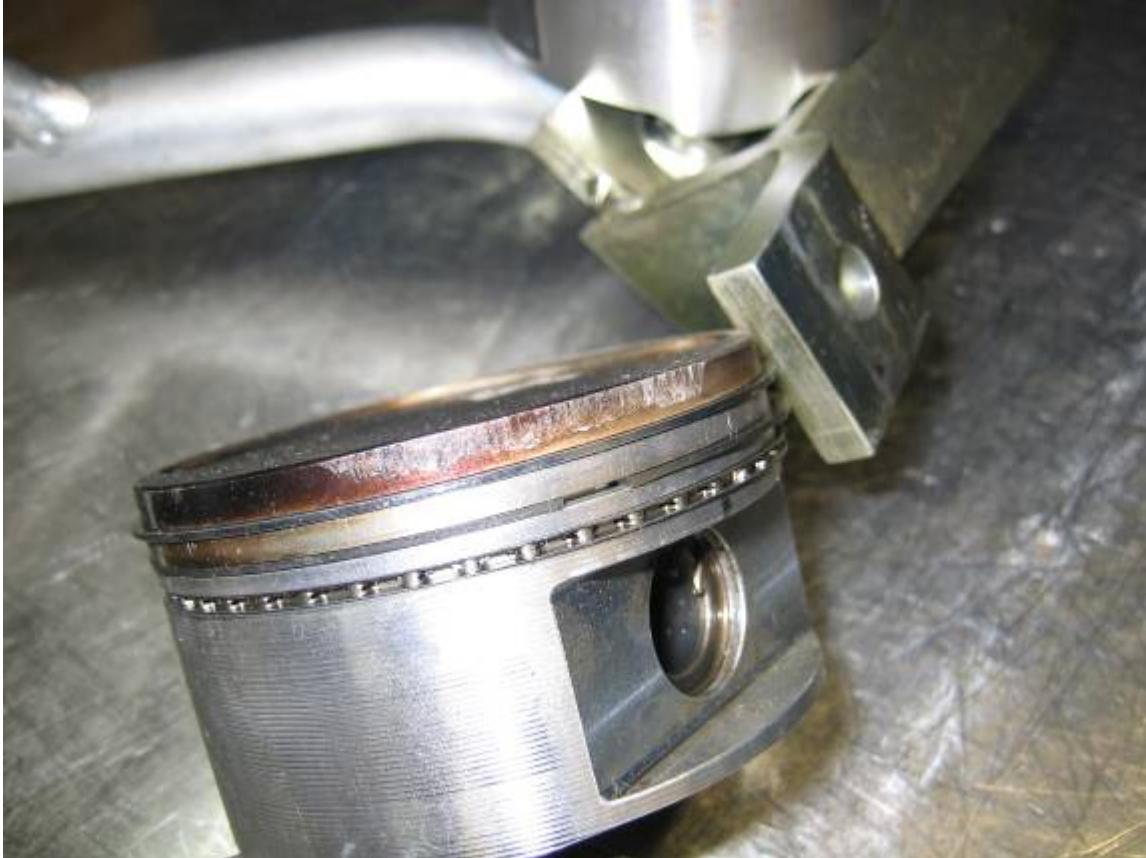
Insufficient Fuel Causing Piston Seizing on Crown
