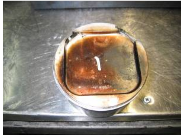
Short Term Catastrophic Detonation
