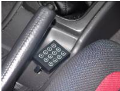
Australian delivered alarm module
