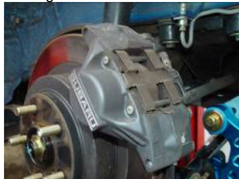
MY03 WRX front calliper, later models and limited editions were painted red
