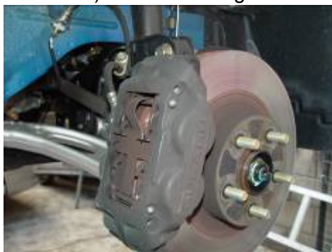
MY03 WRX front calliper, later models and limited editions were painted red
