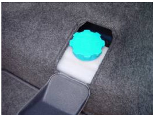
Australian STi water spray tank is in the boot. Controls were simple, with no auto function
