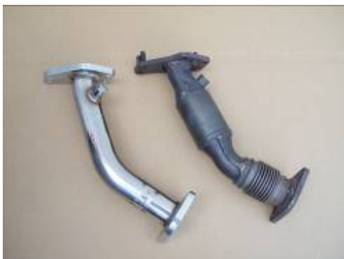
Exhaust up pipe to turbo, note bulge for "pre" cat in OEM part. Factory clock in dash on both sti and WRX
