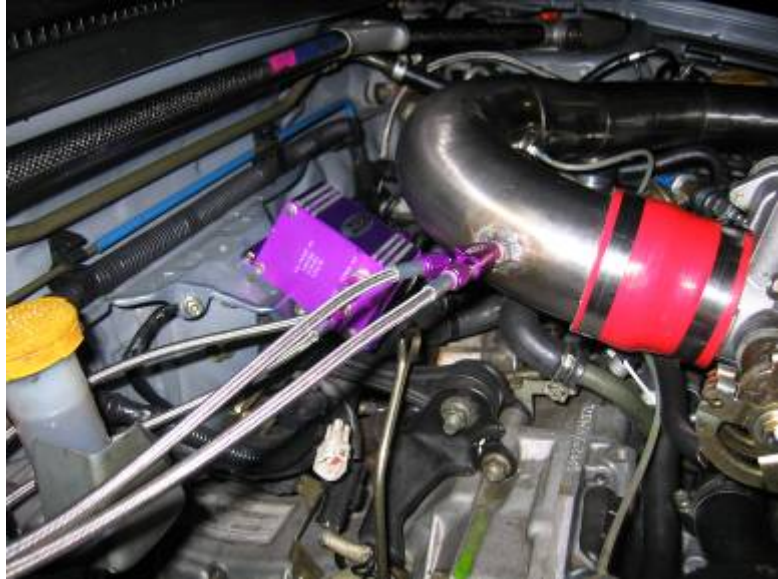
Nos Nozzle In Intake Pipe
