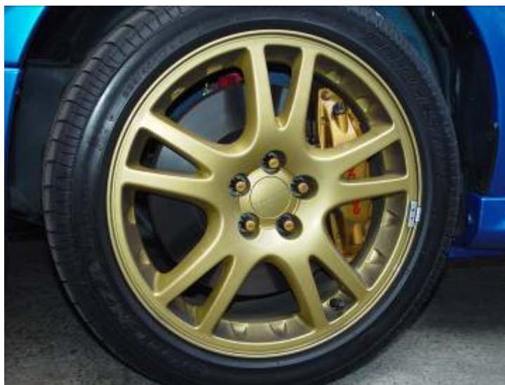
STi MY05 changed to new larger wheel brgs (front) with increased PCD for wheel nuts
