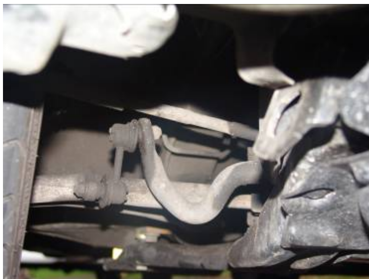
Sedan front suspension, note alloy arm and solid drop link
