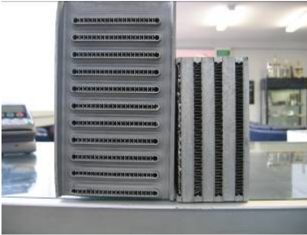
Tube and Fin vs Bar and Plate Core Side View
