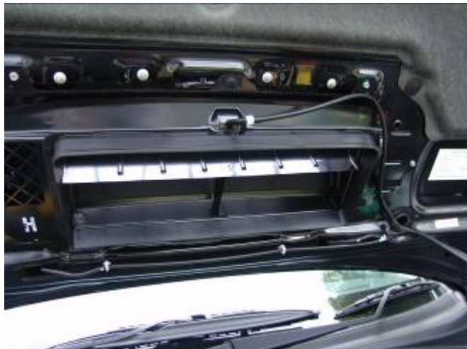
Under side of scoop with air splitter
