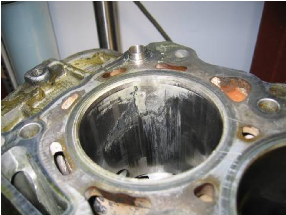
Engine Block Damaged By Detonation
