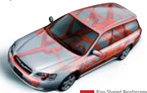
Ring-Shaped Reinforcement Frames
