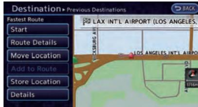
4. The selected destination is displayed at the center of the map. Touch [Start] after confirming the location of the displayed destination. The system sets the destination to the selected location and starts calculating a route.
