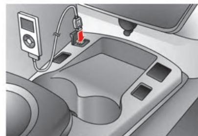
Connect the iPod® cable to the USB connector. If the iPod® supports charging via USB, the battery of the iPod® will be charged while connected to the vehicle.
