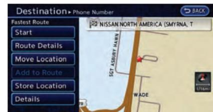
5. The selected destination is displayed at the center of the map. Touch [Start] after confirming the location of the displayed destination. The system sets the destination to the selected location and starts calculating a route.
