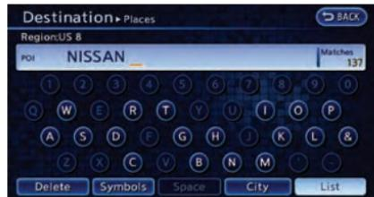
4. Enter the name of the destination facility. After finishing the entry, touch [List]. A list screen is displayed.
