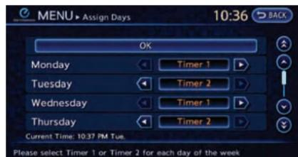
4. To set the A/C-Heater Timer (Climate Ctrl. Timer) for different days of the week, touch [Assign Days]. Either Timer 1 or Timer 2 can be set for each day of the week to operate climate control. After setting, touch [OK]. The previous screen is displayed.
