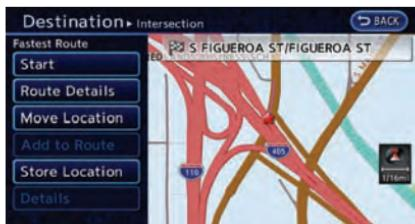
11. The select destination is displayed at the center of the map. Touch [Start] after confirming the location of the displayed destination. The system sets the selected location as the destination and starts calculating a route.
