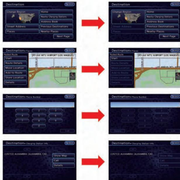
To ensure safe driving, some functions cannot be operated or have limited operation while the vehicle driving is above 5 mph (8 km/h).
