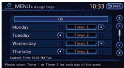
4. To set the timer charge for different days of the week, touch [Assign Days]. Either Timer 1 or Timer 2 can be set to perform battery charging for each day of the week. When the settings are completed, touch [OK].
