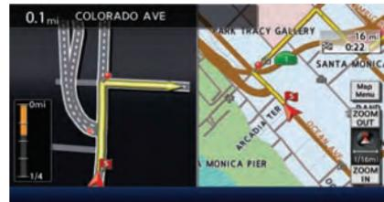
When approaching a guide point, the system automatically changes to the split screen and shows an enlarged view of the intersection on the left screen. To switch to the full screen mode while the enlarged intersection view is displayed, push the **MAP** button. Pushing the **MAP** button again displays the enlarged intersection view.
