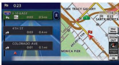
The list screen for showing the guide points to the destination and the map screen can be displayed at the same time. An enlarged intersection view is automatically displayed when the vehicle approaches the guide point.
