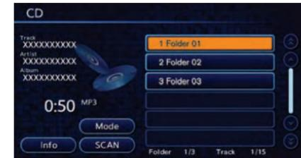
Push the **CD·AUX** button to turn on the audio system and display the audio screen. Push the **CD·AUX** button to toggle the mode: iPod player/USB memory→CD→Bluetooth® streaming audio\*1→AUX.
