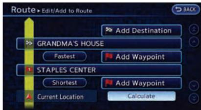
6. By touching [Calculate], the system will recalculate the routes. After the route search is completed, the display will automatically return to the current location map screen.
