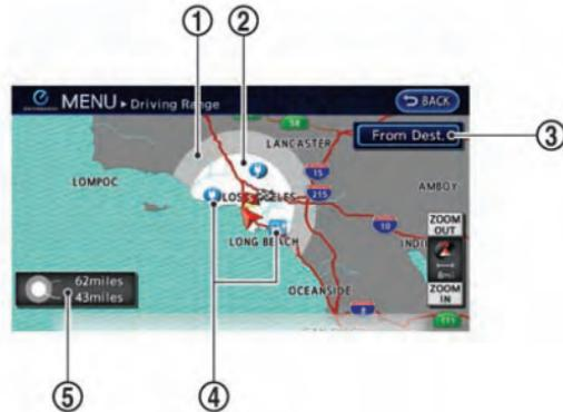
① The extended estimated driving range is displayed using the possible driving distance on the meter as a radius.
