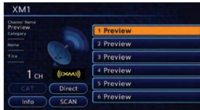
Push the **XM** button to turn on the satellite radio and display the XM satellite radio screen. Push the switch to toggle the radio mode: XM1→XM2→XM3.
