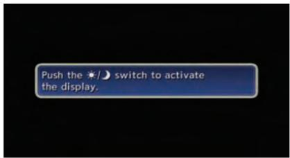
When any button is pushed with the display off, the display turns on. The display will automatically turn off when there is no switch operation for 5 seconds.
