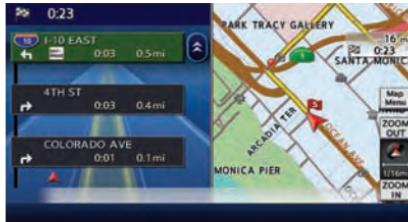
Depending on the setting, the system can constantly display the split screen and show the turn list on the left screen. When approaching a guide point, the left screen automatically switches to an enlarged view of the intersection. To switch to the full screen mode, push the **MAP** button. Pushing the **MAP** button again displays the turn list.
