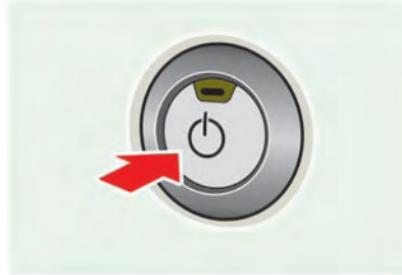
1. The system starts when the power switch is pushed to the "ACC" or "ON" position. The start-up screen is displayed.
