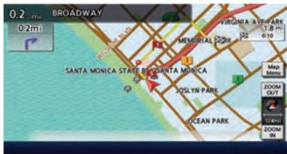
When the **MAP** button is pushed, a map screen where the vehicle position is centered is displayed.
