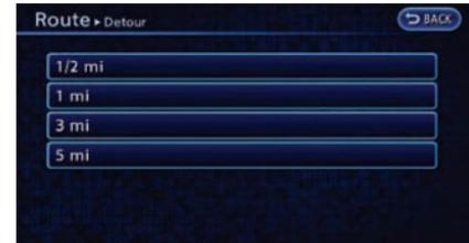
3. Touch a detour distance. After calculating the detour, the system displays the detour route on the map.
